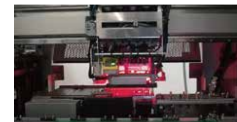
JM-100 placement/No need to replace nozzle
