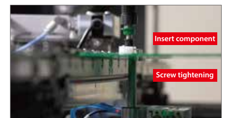
One unit can insert component and screw tightening
