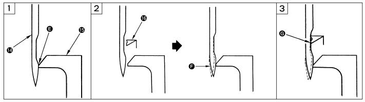
[The standard for adjusting the clearance between the needle and the blade point of the shuttle] Use a standard Schmetz 794-Nm230 needle.
