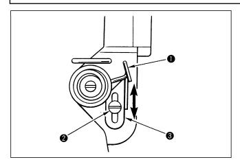
The standard stroke of thread take-up spring **1** is 8 to 15 mm.
