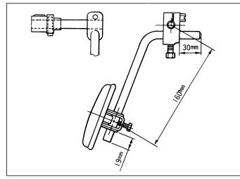
Assemble the knee press plate supplied with the machine as illustrated above.
