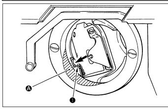
Turn the handwheel by hand (until the needle bar comes down to the lowest point of its stroke) so that case retaining spring
