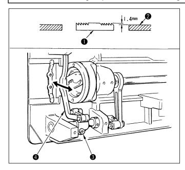
The advance amount of the feed dog from throat plate As already been adjusted to 1.4 mm.
