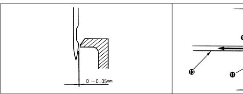
\* Clearance between the needle and the shuttle driver The clearance between the needle and the needle guide of the shuttle driver has already been adjusted to the range of 0 through 0.05 mm.
