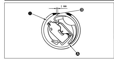
★ The position of the shuttle when it is recessed most. When shuttle ① turns counterclockwise until it will go no further and the shuttle and the shuttle race come in contact with each other at point ③, a distance of 1 mm should be provided between the blade point of the shuttle and end face ③ of the shuttle race.
