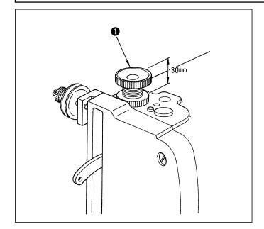
The standard height of presser spring regulator ① 30 mm above the main unit surface.
