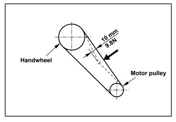
Adjust the belt tension with the height of the motor so that the belt sags 10 mm when the center of V belt is applied with a 9.8N load.
