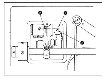
As standard timing of the feed dog, when the center of the needle aligns with the hook with the feed pitch set to "0", the feed dog should move from right to left by 1 mm when observed from the face plate by moving the feed lever from the position to set the normal feed pitch to the maximum value to the position to set the reverse feed pitch to the maximum value.
