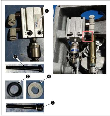
3) Attach the cylinder unit 1 to the arm and temporarily tighten it with 234.
