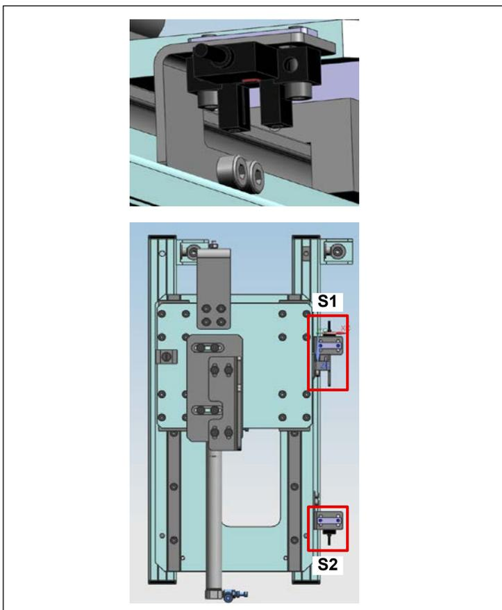
Fix it using screws so that the slit facing the sensor faces downward as shown on the left.
