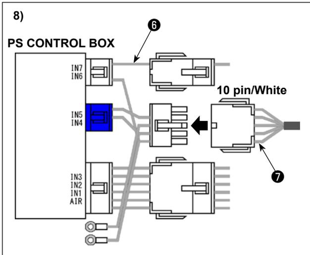
8) Connect control cable 7 of the BK control box to BK10\_RELAY\_CABLE\_ASSY\_A 6 .
