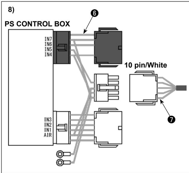
8) Connect control cable 7 of the BK control box to BK10\_RELAY\_CABLE\_ASSY\_A 6 .
