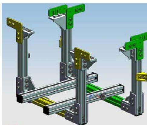
**PS-910-6055 Reference drawing of the completed state of the aluminum frames**
