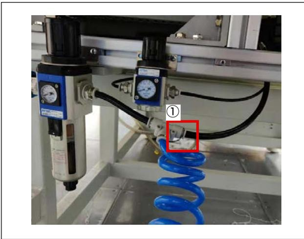
① Detach the air tube that has been connected to the manual valve.
