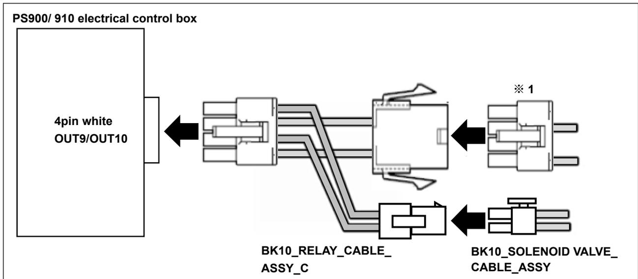
8) Connect the BK10\_RELAY\_CABLE\_ASSY\_C to the electrical control box. Connect the BK10\_RELAY\_CABLE\_ASSY\_C to the BK10\_SOLENOID VALVE\_CABLE\_ASSY.
