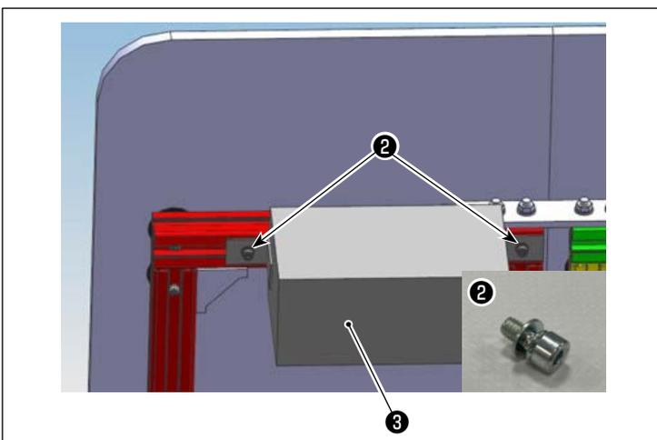
Install control box ③ to the aluminum frame with M4 x 8 screws ② .
