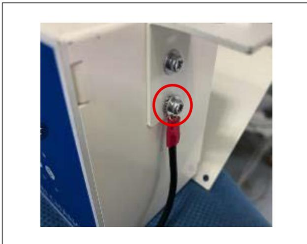
1) Fix a grounding wire to the BK control box with a screw.
