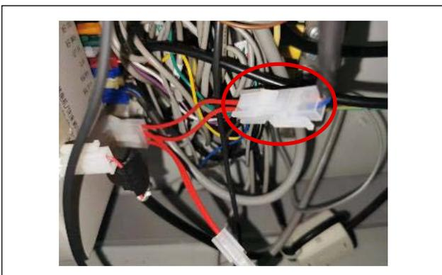
7) Connect the BK10\_SOLENOID VALVE\_CABLE\_ASSY to the BK10\_RELAY\_CABLE\_ASSY\_C coming from the electrical control box.
