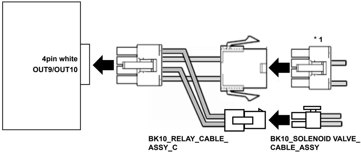
6) Connect the BK10\_RELAY\_CABLE\_ASSY\_C to the electrical control box. Connect the BK10\_RELAY\_CABLE\_ASSY\_C to the BK10\_SOLENOID VALVE\_CABLE\_ASSY.
