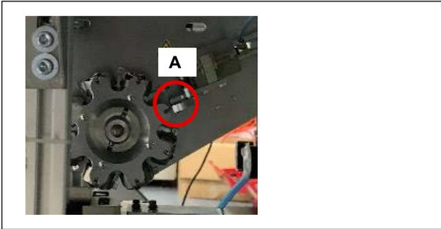
③ At the time of first setup after the power to the sewing machine is turned ON, the chuck stand-by position **A** of the BK should be empty with no bobbin placed on it.
