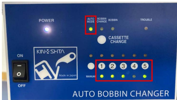
2) Switch the control box to manual mode operation.
