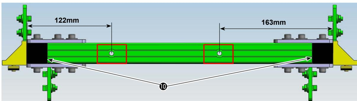
5) Install support aluminum frames (asm.) ⑥ to the sewing machine. Secure link plates (B) ⑪ (four sets) to the aluminum frames of the main body of the sewing machine in prior.
