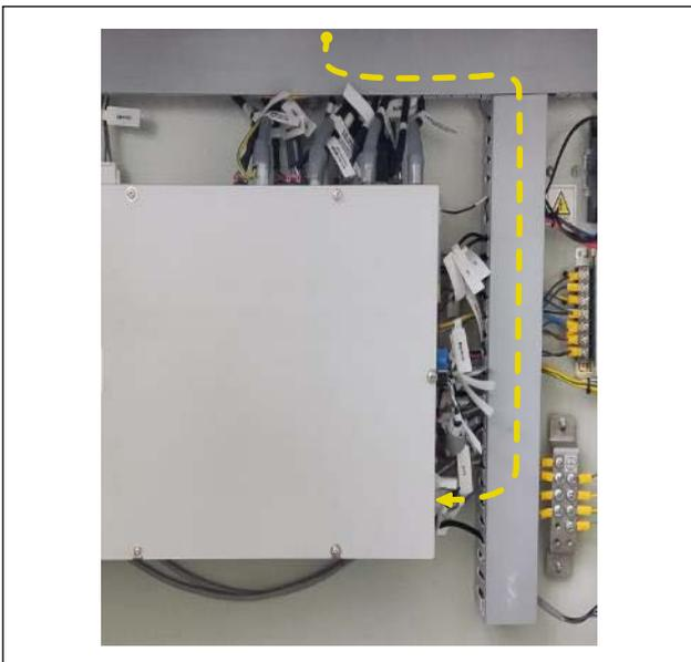
6) Wire the BK10\_SOLENOID VALVE\_CABLE\_ASSY as shown in the figure.
