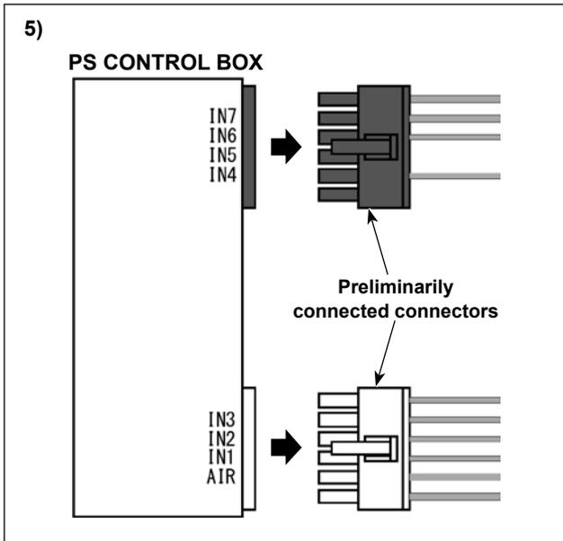
5) Remove the connectors (12-pin/black and 12-pin/white) that have been preliminarily connected to the side face of the electrical control box.
