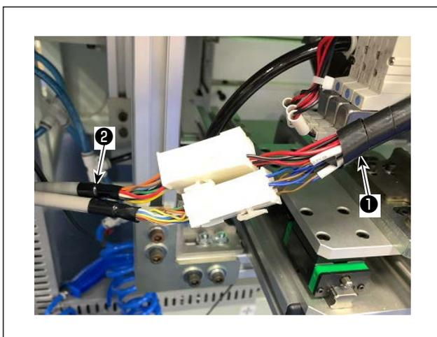
1) Connect the connectors of the cylinder sensor and solenoid valve cable ① on the BK main unit side to the connectors of the cylinder sensor and solenoid valve cable ② on the BK-10 control box side.
