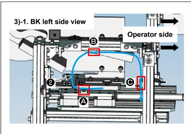
3) Wire the cylinder sensor and solenoid valve cables ② on the BK control box side according to the route indicated by the blue arrow in the figure. Fix them with a fixing base and a cable clip band at the positions ① and ② along the way.
