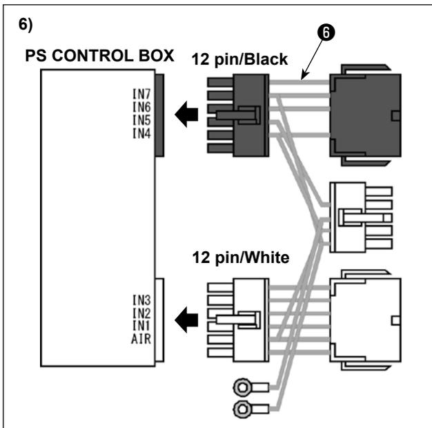
6) Connect the connectors (12-pin/black and 12-pin/white) of BK\_RELAY\_CABLE\_E\_6055 6 to the electrical control box.
