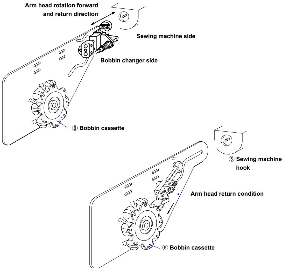
**Caution** When pressing the arm head key ⑩, be sure to move the bobbin changer feed base toward the operator side.
