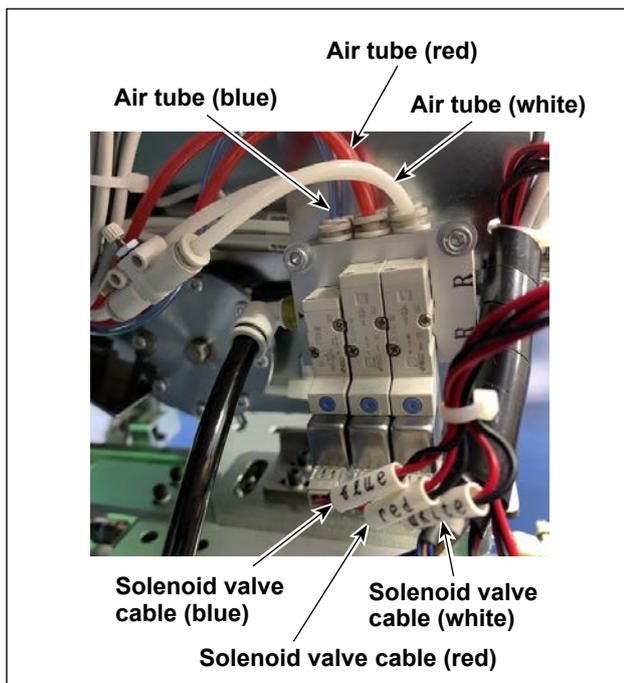
1) Connect the solenoid valve cable according to the color of the solenoid valve air tube of the main body of the bobbin changer.
