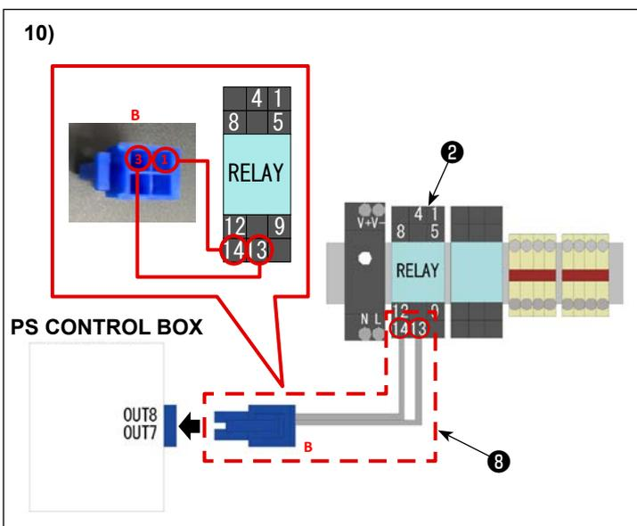
10) Connect the connector of BK10\_RELAY\_CABLE\_ASSY\_B 8 to the connector (4-pin/blue) of the OUT7/OUT8 of the electrical control box. Connect the ring terminal of BK10\_RELAY\_CABLE\_ASSY\_B 8 to RELAY TERMINAL 2 .
