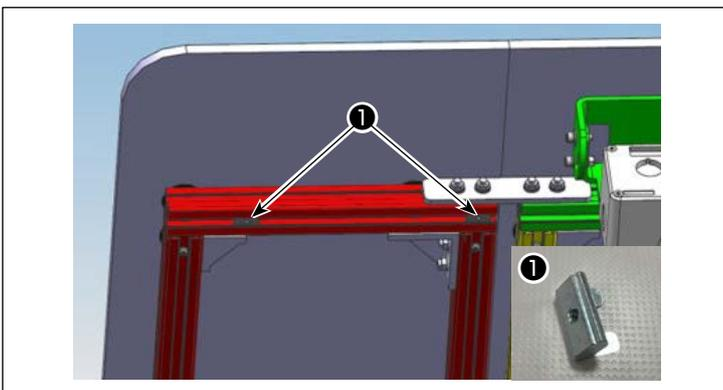
Insert two M4 special nuts ① in the aluminum frame of the 6055 auxiliary table.
