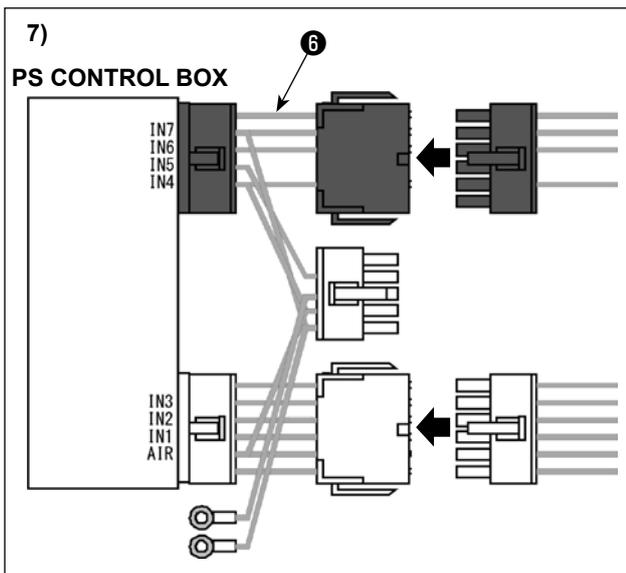
7) Connect the connectors you have removed from the electrical control box in Step 5) to BK\_RELAY\_CABLE\_E\_6055 6 .
