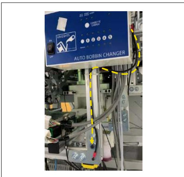
2) Wire the grounding wire as shown in the figure. Secure the ring terminal to the sewing machine frame with a screw.
