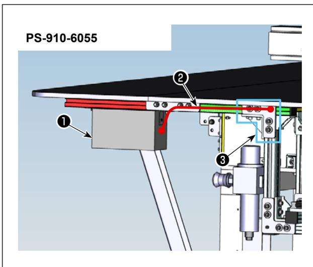
2) Wire the ground wire ② attached to the BK control box ① as indicated by the arrow in the figure, and use the screw holes in the L link plate ③ to fix it with screws.
