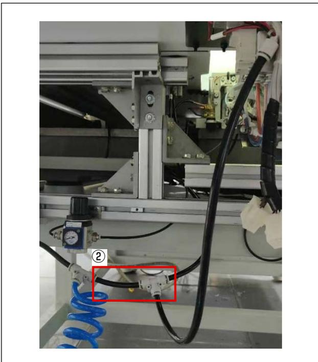
② Connect the air tube (100 mm: 1 piece) coming from the BK-10 and the T-shaped union as shown in the figure.
