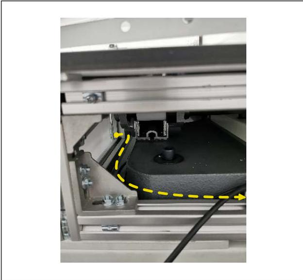
4) Wire the solenoid valve cable according to the route shown in the figure.
