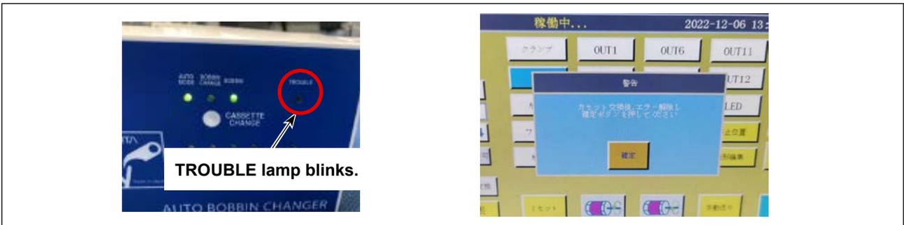
① Remove the cassette that has been placed on the main body of the BK without turning OFF the power to the sewing machine and BK control box.
