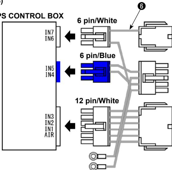
6) Connect the connectors (white/6-pin, blue/6-pin and white/12-pin) of BK10\_RELAY\_CABLE\_ASSY\_A ⑥ to the electrical control box.
