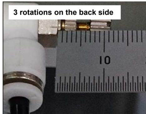
If an error recurs after you have adjusted the speed controller as described above, adjust the speed controller so that approximately six seconds are required from the moment the lengthwise feed base starts to retract to the moment the arm goes up.
