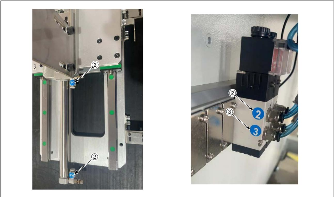
Fix the air tube to the aluminum frame with fixing bases and cable clip bands.
