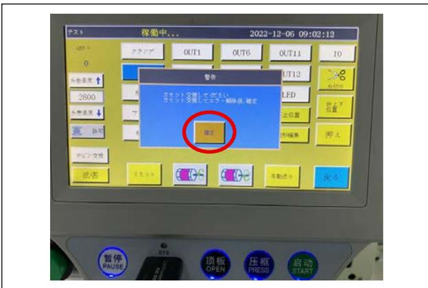
⑤ A message is displayed on the operation panel of the sewing machine. Press the "Enter" button.
