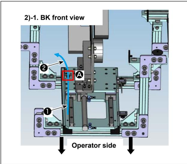
2) Wire the cylinder sensor and solenoid valve cables ② on the BK control box side according to the route indicated by the blue arrow in the figure. Fix them with a fixing base and a cable clip band at the position ① along the way.
