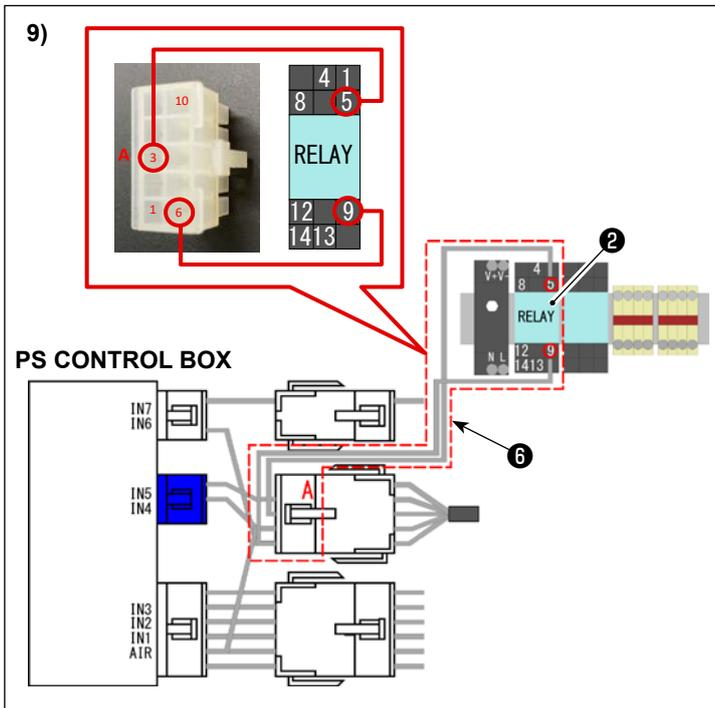
9) Connect the ring terminal of BK10\_RELAY\_CABLE\_ASSY\_A 6 to RELAY TERMINAL 2 .
