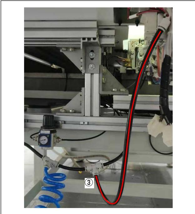
③ Connect the air tube (500 mm: 1 piece) coming from the BK-10 to the T-shaped union and the union on the BK main unit side as shown in the figure.
