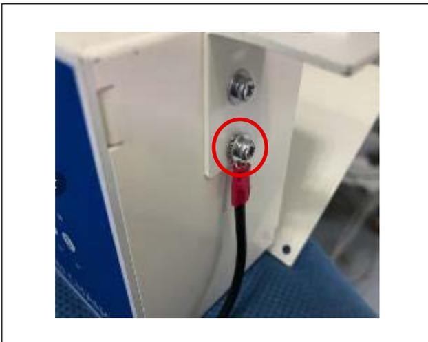
1) Fix a grounding wire to the BK control box with a screw.
