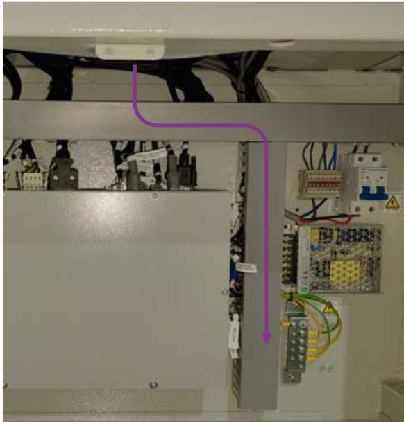
5) Wire the BK10\_SOLENOID VALVE\_CABLE\_ASSY according to the route indicated by the arrow in the figure.
