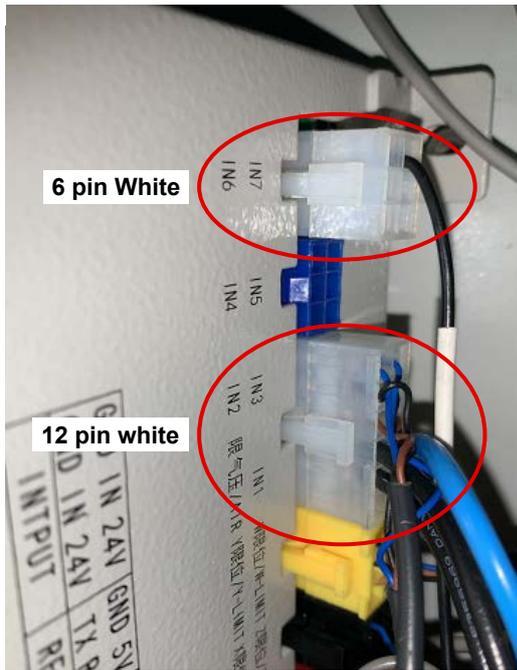
5) Remove the connectors (6-pin/White and 12-pin/White) that have been preliminarily connected to the side face of the electrical control box.
