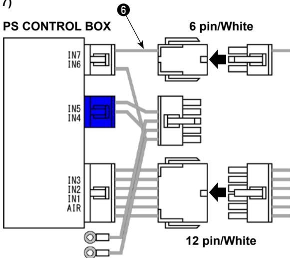
7) Connect the connectors that you have removed from the electrical control box in Step ⑫ to the BK10\_RELAY\_CABLE\_ASSY\_A ⑥ .
