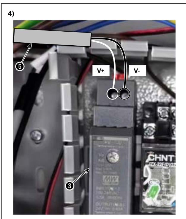
4) Connect power cable ❺ of the BK control box that you have drawn into the electrical rack in Steps ❹ to ❸ to BK10\_24V\_POWER\_SUPPLY ❸ .
