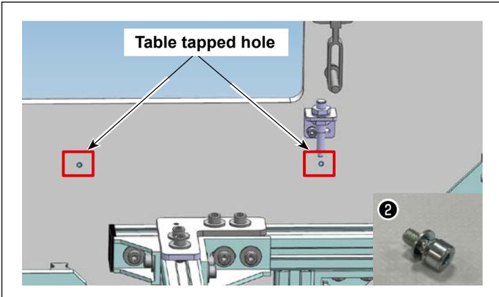
Install control box ① to the front center table of the sewing machine with M4 × 8 screws ② (two pieces).
