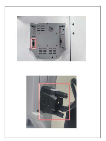
3) Connect the barcode reader plug to the connector at the panel as shown.
