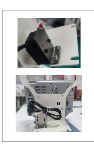
4) Pass the cable clip band **7** through this hole in the barcode reader mounting plate and fix the cable behind the panel.
