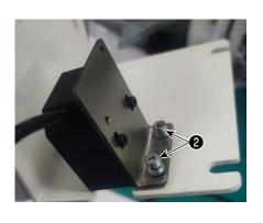
2) Remove the panel mounting plate fixing screws 3 and 9, and fix the barcode reader mounting plate 1 and the panel mounting plate with the screws 2.
