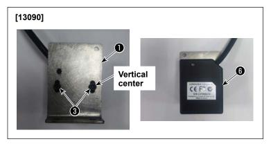
1) Fix the barcode reader 6 and the mounting plate 1 with the screws 3.
