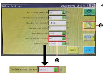
4) To allow the barcode reader to recognize the template, change from "Electronic identification label" to "Barcode". Then, press .
