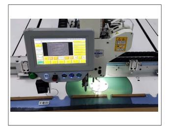
2) Place the barcode seal in the cassette right under the barcode reader.
