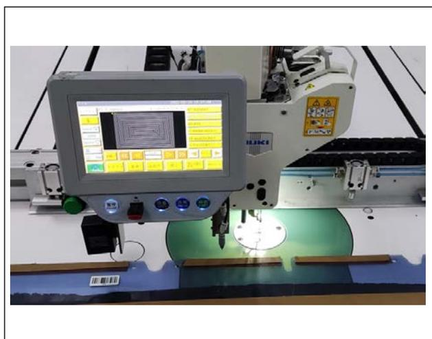
2) Place the barcode seal in the cassette right under the barcode reader.
