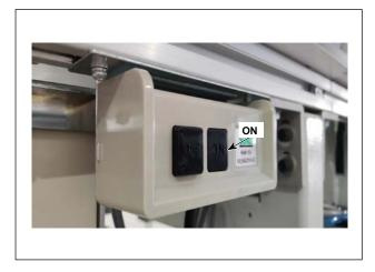
1) The blower operates when the power supply for the blower is turned ON.
