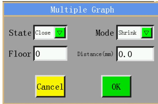
**State**  : State ON/OFF. Determine whether multi-curve sewing is employed or not for next capture.
