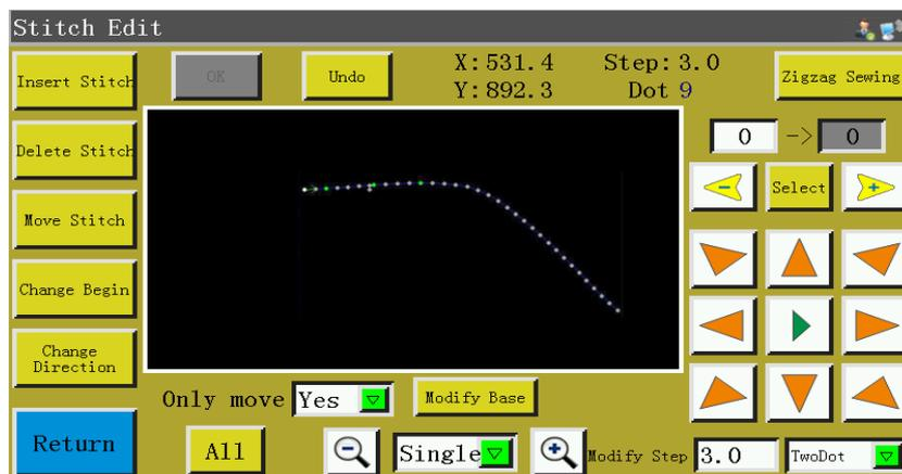
A certain needle point can be added, deleted, translated or changed. (When a point turns green, it means the function code has been assigned to that point)
