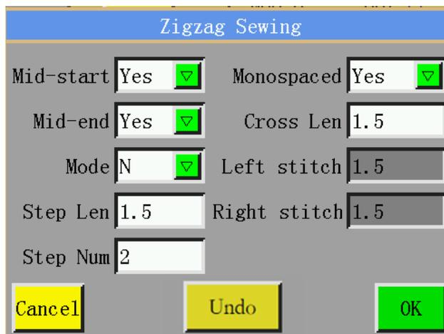
Set up the parameters of zigzag stitch,
