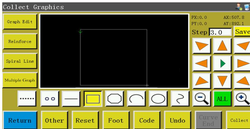
In the case of rectangle capture, two points with different X and Y coordinates generate a rectangle.
