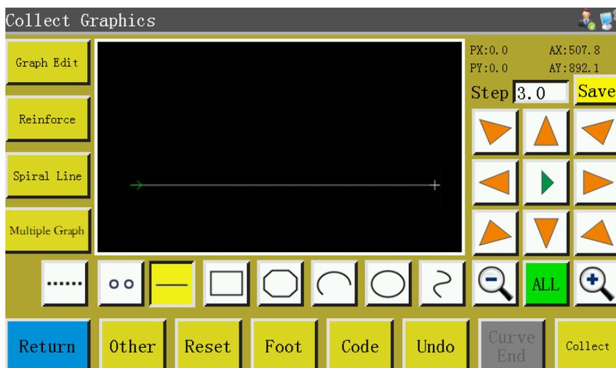
In the case of straight line capture, two points generate a segment of straight line.
