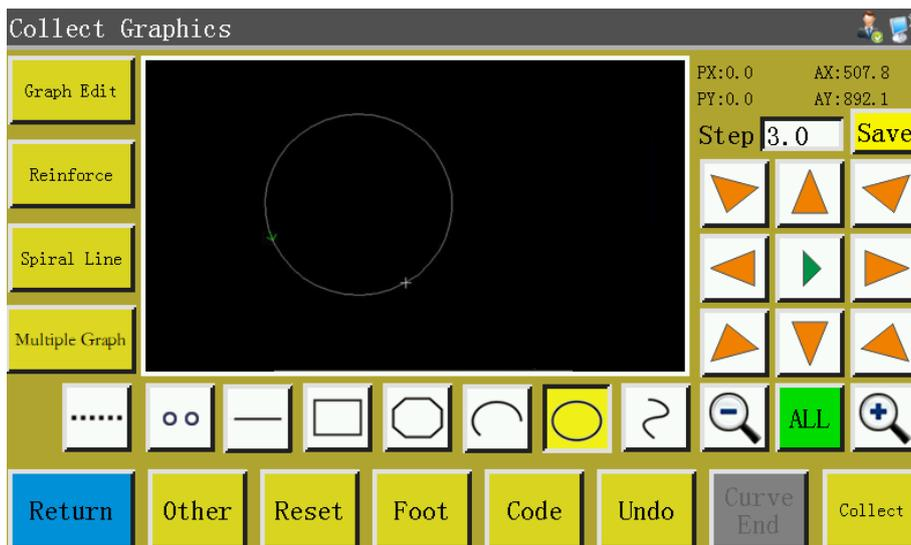
In the case of circle capture, any 3 points that are not in the same straight line generate a circle. The processing sequence: The first point (start point) > The second point > The third point > The first point (end point).
