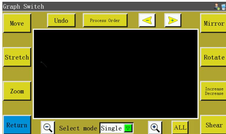
**Stretch**: Select the graph to be handled, set the horizontal-to-vertical ratio of the curve, and click “OK”, when the graph will be stretched based on the set parameters.
