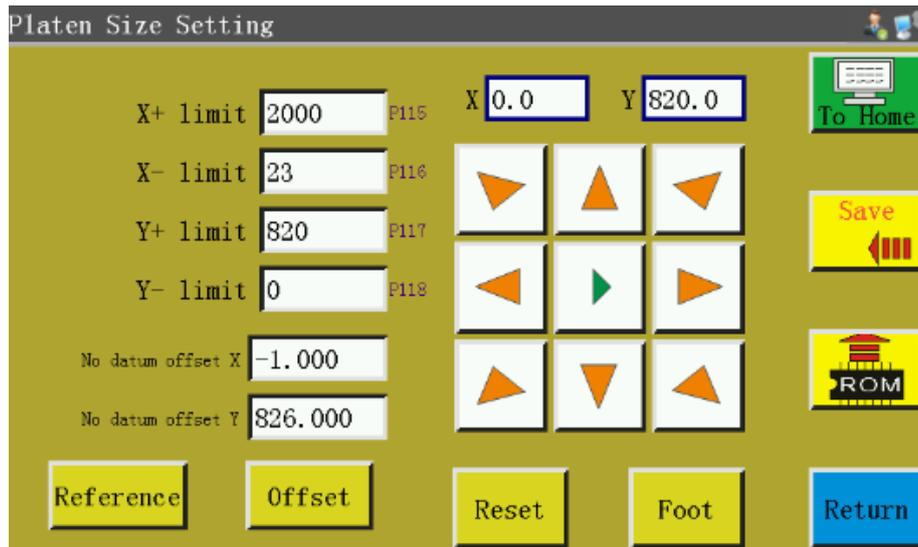
**Reference** : When adjusting the offset-free reference point, the offset reference point should be set first.
