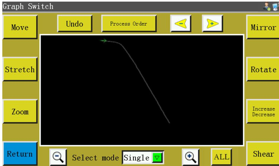
This graph can be changed or edited by setting up parameters such as pan, stretch, scale, rotation, mirroring, increase/decrease, and shear.
