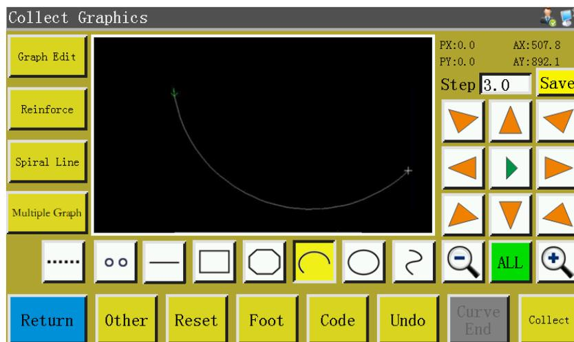
In the case of arc capture, any 3 points that are not in the same straight line generate an arc: The first point is the start point of arc, the second point being the height reference point of arc, and the third
