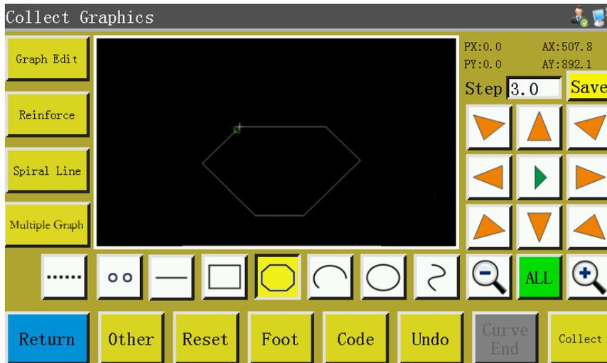
In the case of polyline segment capture, up to 127 consecutive points can be handled, and the line segment will be generated by two points determining straight line.
