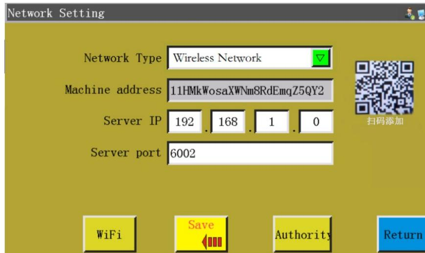
Device address: Show the unique address code of current device. The companion APP "Xing Huo IoT" can be used to scan the QR code address of this interface to add the device to the APP for device management.
