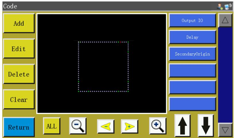
The graph is displayed in the form of needle points in this interface; select the position you want to edit (when a certain needle point turns red), when function codes can be added, edited, deleted and removed at the location of that needle point. When a function code is assigned to a certain point, that point will turn green. Click on this point, when the set function code appears on the right.
