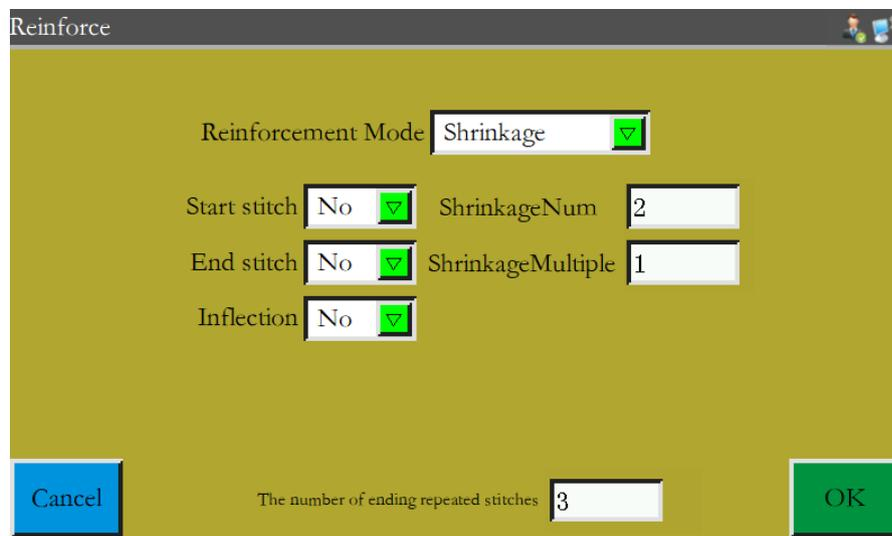
The number of ending repeated stitches 3 : Repeated stitches are required at the end of the line
