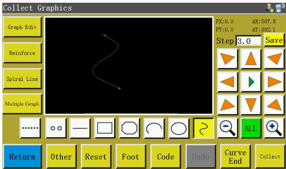
In the case of curve capture, up to 127 consecutive points can be handled, and the Bezier is generated by the degree of arc of the neighboring 4 points. The capture point shall be as dense as possible at the turning so as to achieve optimal curve effect. The capture of less than 3 points can generate curve.
