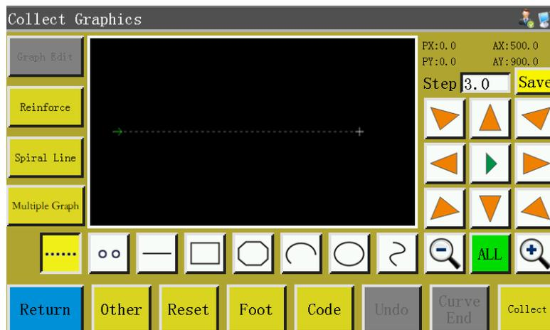
In the case of idle capture, two points generate an idle segment.
