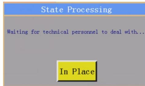
Upon the arrival of technician at the equipment, he/she can click **In Place**, when the machine status displayed on console reads "Waiting for solution". When **Close Case** is clicked after the removal of anomaly, the machine status displayed on console returns to normal.
