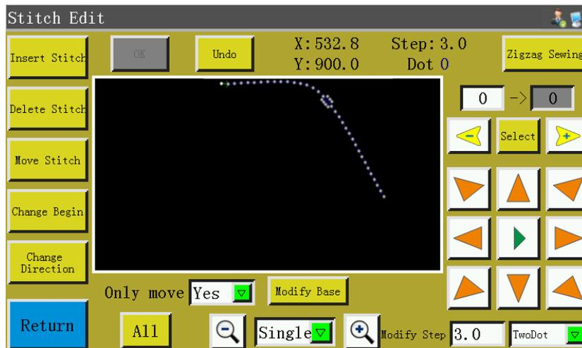
**Node Edit** : The entire curve is presented in the form of many nodes so that the curve can be changed by adding, deleting and translating the nodes. Moreover, even the start point and the direction of the entire curve can be changed (the key operation mode is the same as needle point editing). The interface is as follows:
