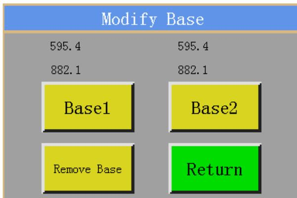
Modify Base: Set the current selected pin point as the reference point of the graph, the reference point 1 as the reference point 1, the reference point 2 as the reference point 2, and the clearance reference point to clear all the reference points that have been set.
