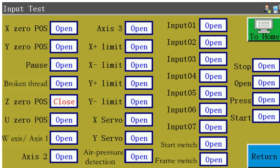
You can manually trigger relevant sensors and check whether the input status has changed, and determine if the sensor or hardware is in good condition.
