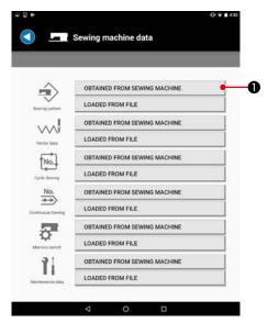
1) Press the "OBTAINED FROM SEWING MACHINE" button **1** of Sewing pattern.
