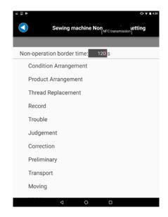
Set the non-operation boundary time and the order of non-operation items on the non-operation setting screen of sewing machine.
