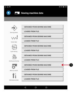
1) Press the "OBTAINED FROM SEWING MACHINE" button **1** of Memory switch.
