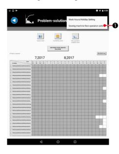
1) Select the "sewing machine on-operation setting" **1** menu from the menu displayed at the upper right section of the screen.
