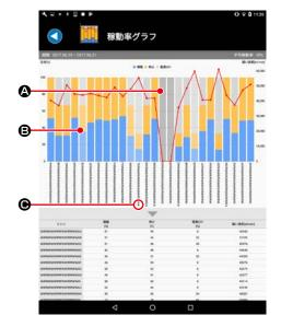
2) The availability chart (current day) is displayed. Progress of the operation status and the average sewing speed can be viewed in the availability chart (current day). The operation rate is totalized taking the period of time to be elapsed from the starting time of the workday (\*1) to the time at which the last data of the day is acquired as 100 %.
