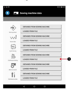
1) Press "LOADED FROM FILE" button **1** for the continuous sewing data.
