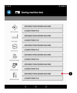
1) Press the "OBTAINED FROM SEWING MACHINE" button **1** of Maintenance data.
