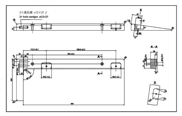
2.03 台板开槽部位尺寸 Size of slotting part of the platen
