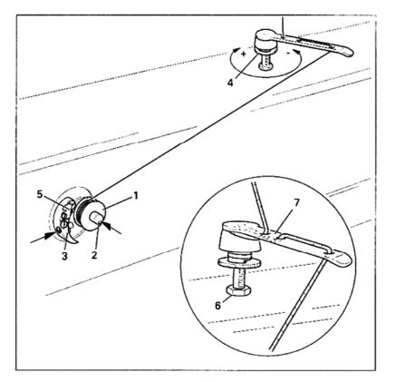
Winding the bobbin thread ,adjusting the thread tension.
