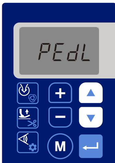
5. When you turn ON the power to the sewing machine while the full automatic mode is set selected, "PEDL" will be displayed on the operation panel as shown in the figure on the left.
