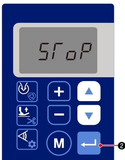
When you depress the back part of the pedal during sewing, the sewing machine stops and the characters [SToP] appear on the operation panel. (D), (E)
