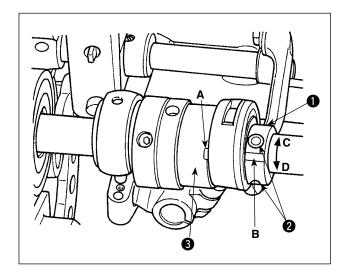
Notch A in collar 3 aligns with notch B in the puller eccentric cam when the roller is placed in the standard position. When changing the feed timing, loosen two setscrews 2 in puller eccentric cam 1 to adjust. When the cam is moved in the direction of C, the start of the roller is advanced, and when it is moved in the direction of D, the start of the roller is delayed.
