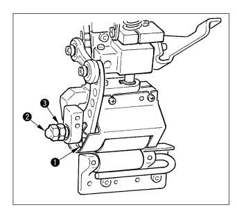
Adjustment is performed with clutch tension spring ① so that the top roller does not overrun at high-speed rotation. When performing the adjustment, loosen cap nut ②, and turn nut ③ to the right (clockwise) to increase the spring pressure. When decreasing the spring pressure, turn nut ③ to the left (counterclockwise).
