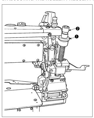
Loosen nut ①, and turn presser spring regulator ② to the right (clockwise) when increasing the presser pressure.
