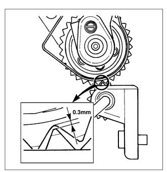
In case of the gear type roller, loosen nut ② and adjust the length of screw ① so that the clearance between the top and the bottom rollers is approximately 0.3 mm in the state that the rollers are lowered.
