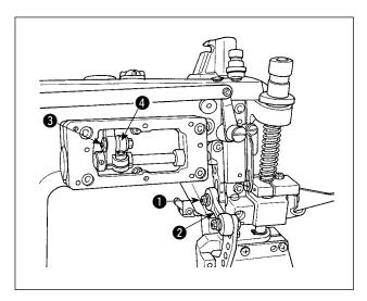
Loosen screw ① when adjusting the feed amount of the roller. Feed amount is decreased when link ② is lifted. Feed amount is increased when link ② is lowered. When changing the feed amount further, loosen screw ③ to adjust. Feed amount is decreased when rod ④ is lifted. Feed amount is increased when rod ④ is lowered.
