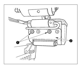
Install rear roller asm.  $\ensuremath{\mathbf{Q}}$  which is contained in the accessories with two screws  $\ensuremath{\mathbf{0}}$ .
