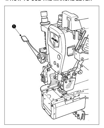
Lift lever **1** when the cloth puller device is not used at the time of performing setting of material or removing material which has been sewn.
