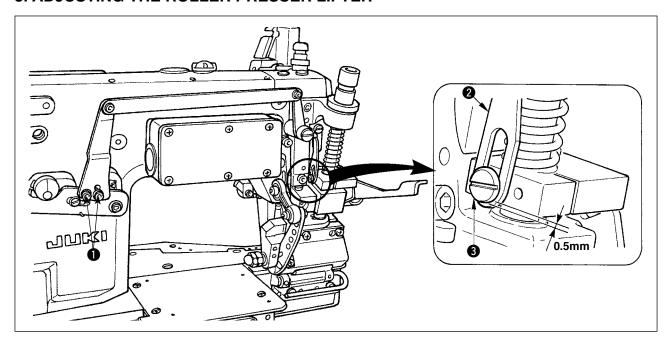
Adjust with two screws **1** so that the clearance between presser lifter lever link, short **2** and hinge screw **3** is 0.5 mm when performing the presser lifting in the state that the top roller is lowered.
