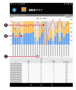
2) The availability chart (current day) is displayed. Progress of the operation status and the average sewing speed can be viewed in the availability chart (current day). The operation rate is totalized taking the period of time to be elapsed from the starting time of the workday (\*1) to the time at which the last data of the day is acquired as 100 %. (Excluding the work break)
