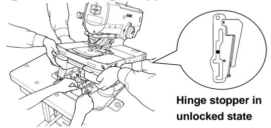
Hinge stopper in unlocked state
