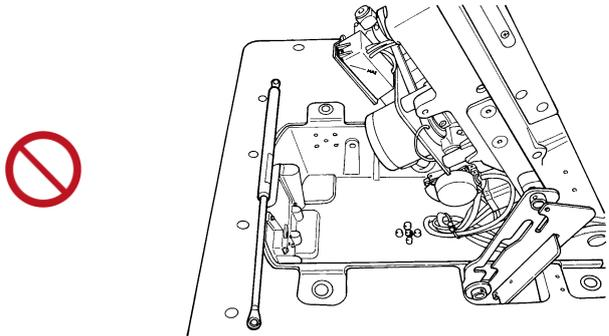
Be sure to check the function of the gas spring periodically. If any functional decline of the gas spring is detected, be sure to replace it with a normal one before using the sewing machine.
