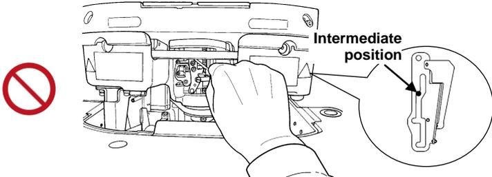
Be sure to lift up the sewing machine until the hinge stopper is locked at the **threading position** to secure the sewing machine.
