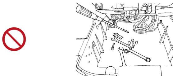
Be sure to make sure that there is no tool or part inside the bottom cover before returning the sewing machine to its home position.
