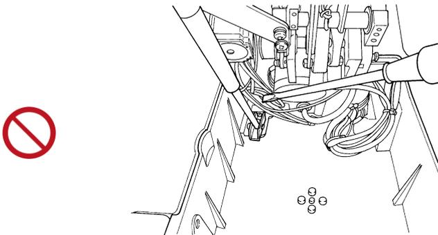
**Do not return** the sewing machine **to its home position with a tool or part placed** inside the bottom cover.
