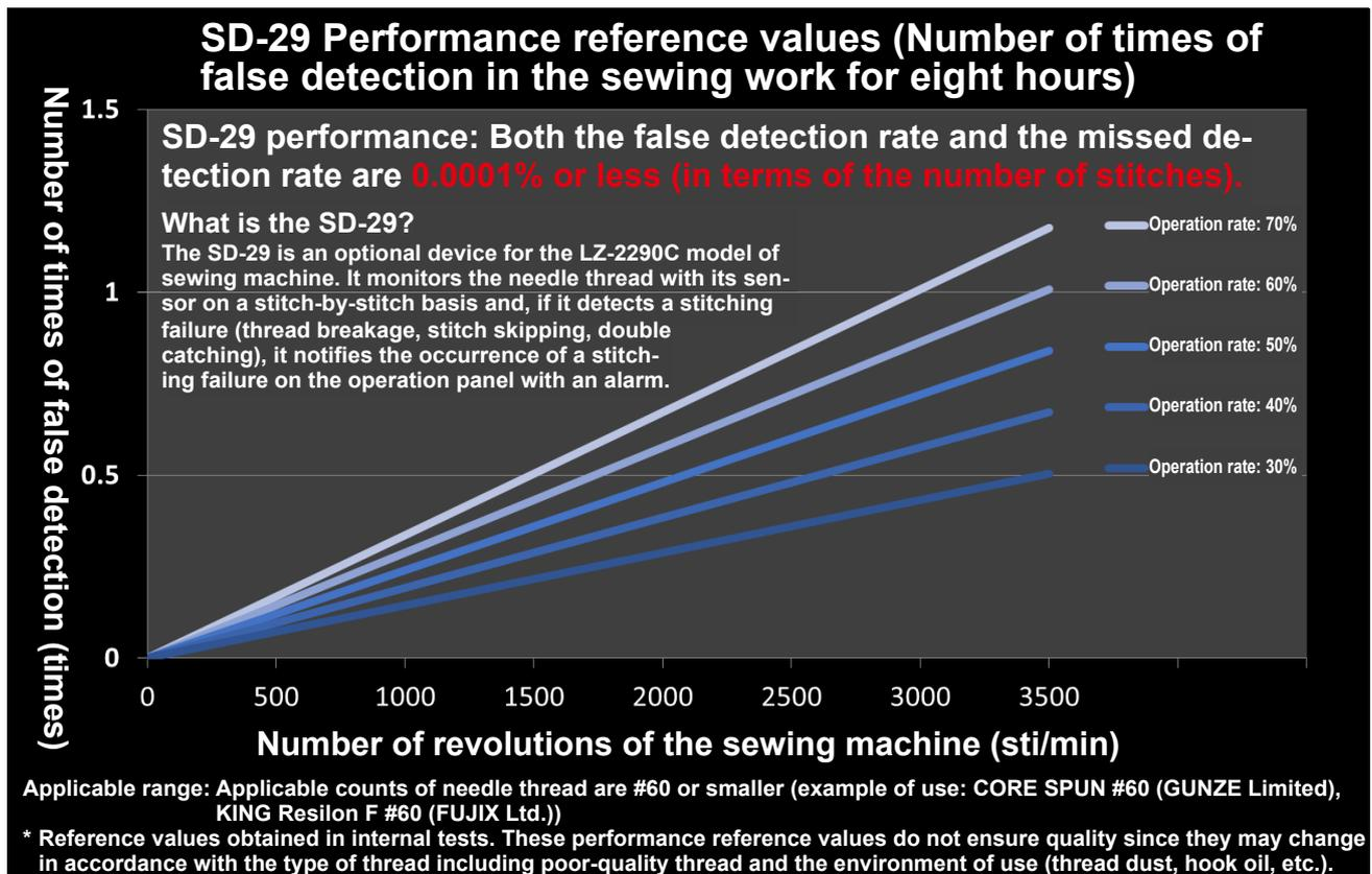
Since this device gives priority to prevention of missing of a stitching failure, it detects an error when the sewing machine falls into the state that is close to a stitching failure.
