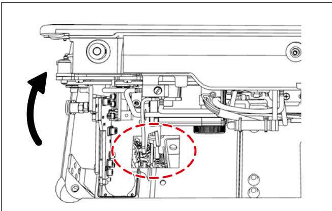
1. Do not raise the main body of sewing machine with the jig placed on the under cover.
