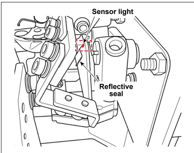
Check to make sure that the sensor light does not hit the reflective tape of the reflective plate when the bobbin case is not attached.
