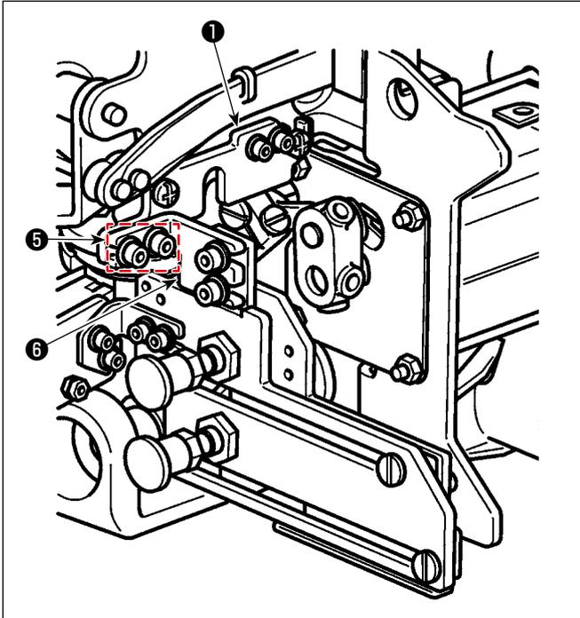
2) Install position adjustment plate C **6** to base plate **1** with setscrews **5** of the position adjustment plate C.
