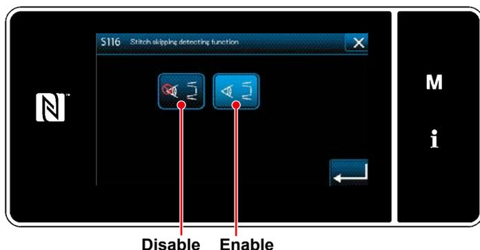
If you want to use the SD-29's detecting function, set "S116 Stitch skipping and double catching detecting function" to "Enable".
