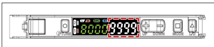
3. Lift the operation plate and lock the index plunger. Check that the light quantity displayed on the amplifier is "9999".
