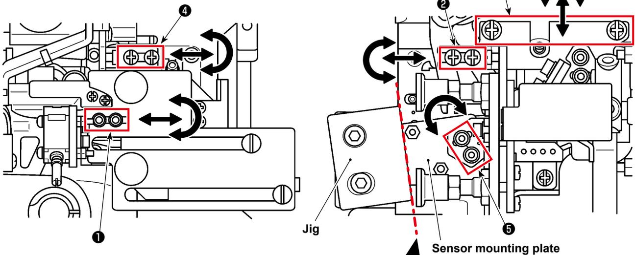
Only as a guide, assemble the jig and the sensor mounting plate so that they are positioned to have an equal clearance of 1 mm over the length (in parallel with each other).
