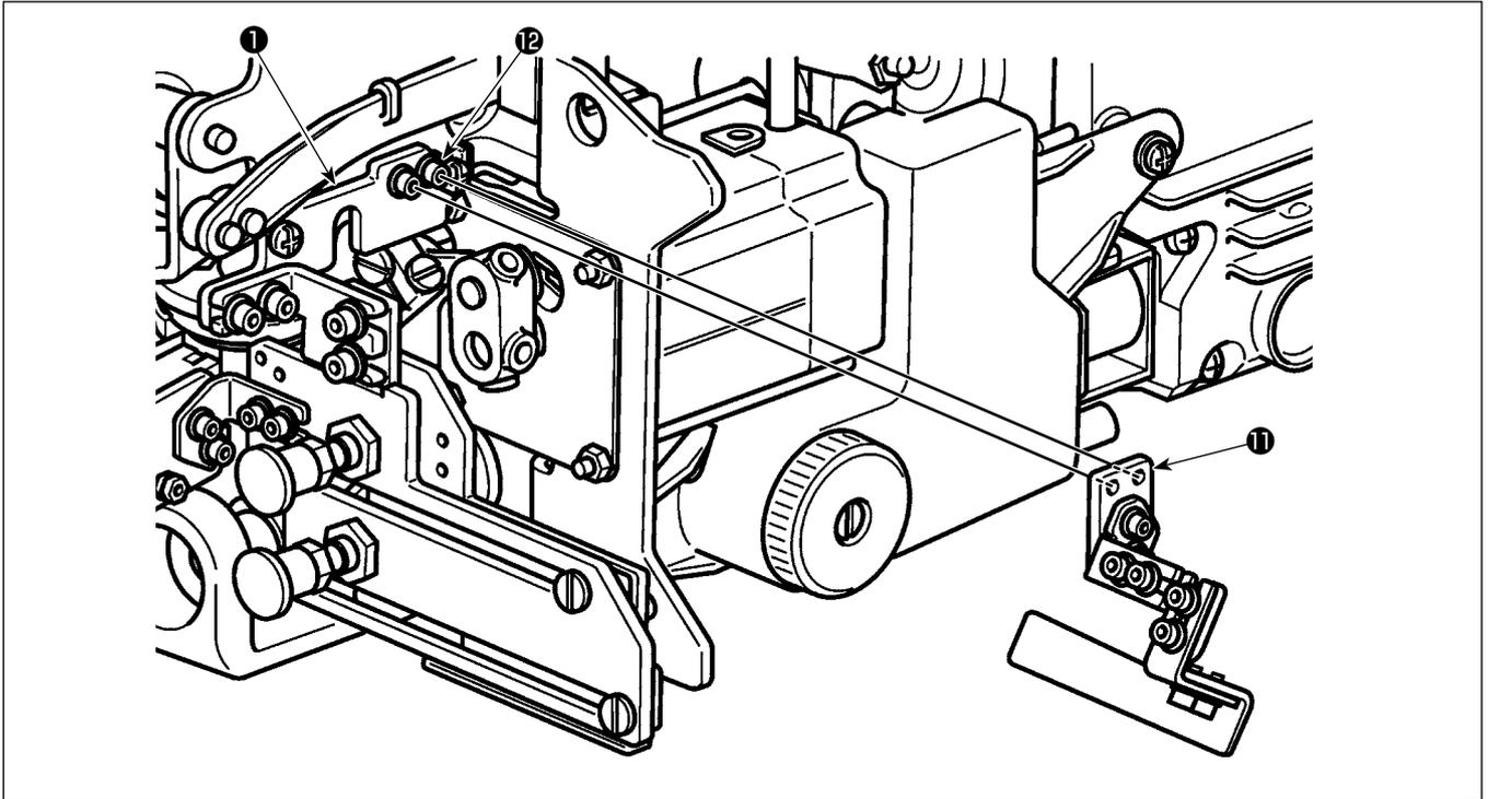
1) Install reflective plate asm. ⑪ to base plate ① with setscrews ⑫ of the reflective plate asm.
