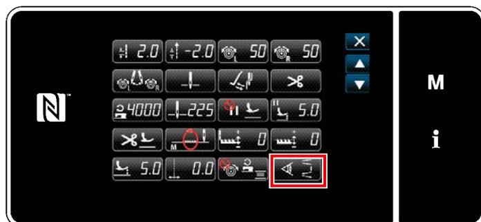
Enable/disable of the stitch skipping detection can be set on a pattern-by-pattern basis.
