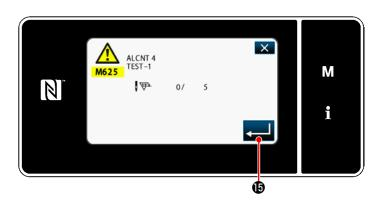
19) When is pressed, the operation is confirmed. Then, the screen returns to the "maintenance management screen".
