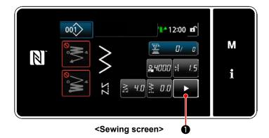
When **1** is pressed on the sewing screen, the "second sewing screen" is displayed.
