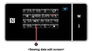
When 4 is pressed, the "Sewing starting position selection screen" is displayed.
