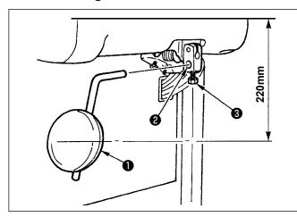
Insert knee-lifter into attaching hole ② and tighten it with bolt ③.
