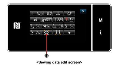
When size of is pressed, the "Sewing starting position selection screen" is displayed.
