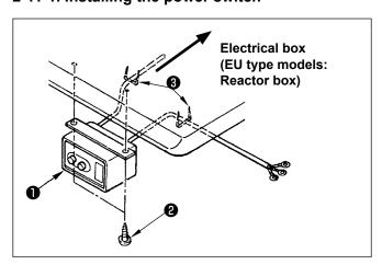
Fix power switch **1** under the machine table with wood screws **2**.
