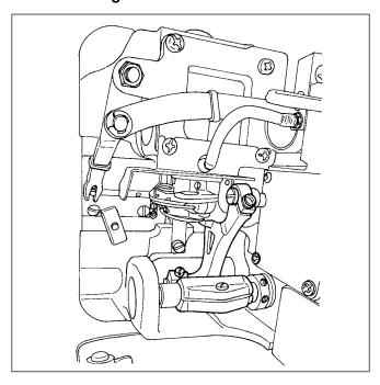
When cloth waste or the like gathers around or adheres to the hook section, trouble (defective sewing, seizure of hook, etc.) of sewing machine will be caused. Periodically clean the section.
