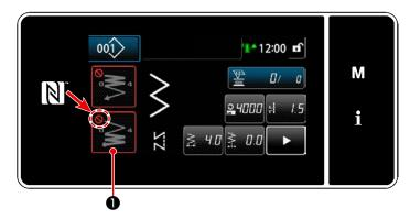
The sewing-end reverse feed stitching pattern can be operated when the sewing-end reverse feed stitching function is placed in the ON state (\infty mark is not displayed).
