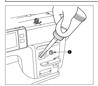
Fill the oil tank with oil before operating the sewing machine.
