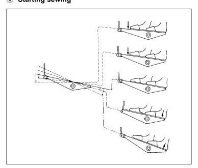
When you depress the pedal, the sewing machine starts sewing.
