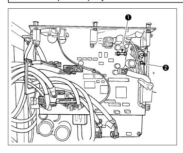
The machine uses the following two fuse. Both are the same fuses.
