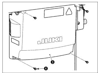
3) Install control box cover **3** with four setscrews **4**.
