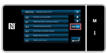
Select the function item to be assigned to the switch. Then, select the input signal status
