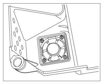
The cooling fan may not produce a sufficient cooling effect on the sewing machine head if cloth chips, etc. have gathered in the cooling fan unit that is installed on the bottom of underside cover.
