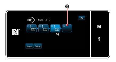
7) In the case a step can be additionally registered to a sewing pattern, step **②** which is not yet set is displayed in the last field.
