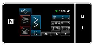
While the one-touch type changeover is being carried out, the object data display is changed, and the one-touch type changeover icon is displayed on ①.
