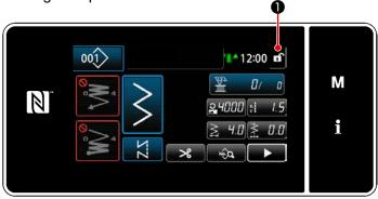
Simple lock is activated by keeping • • held pressed for one second on the sewing screen. Pictograph display • will be as shown below:
