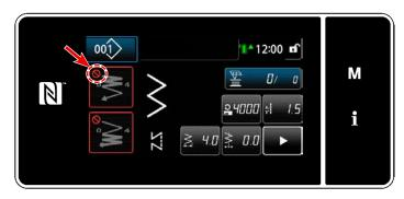
The sewing-start reverse feed stitching pattern can be operated when the sewing-start reverse feed stitching function is placed in the ON state (\infty mark is not displayed).
