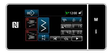
Three different types of the counter are available, i.e., the bobbin thread counter, the sewing counter and the pitch time counter.
