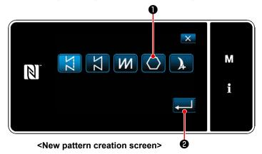
Referring to ② in "8-1-1. Creation of a new pattern" p. 118, select polygonal-shape stitching pattern ① ① on the sewing pattern selection screen. Then, press ② .
