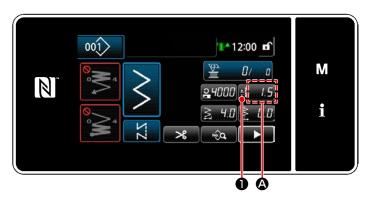
Stitch length is displayed in section **(A)** on the panel. (Example of display: 1.5 mm)
