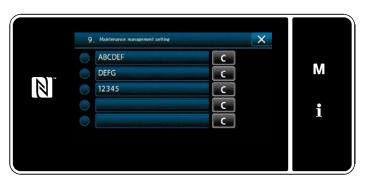
When the counter for which the set value for warning is selected, the "warning counter setting screen" is displayed.
