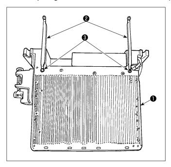
1) Underside cover ground wires ② are attached to the underside cover. Secure underside cover ground wired ② on electrical box ① with screws. At this time, remove once the mounting screws from the underside cover. Install the electrical box to the frame located behind the electrical box in the upward direction as shown in the figure. Use mounting screws ③ that has been preliminarily attached to the frame.
