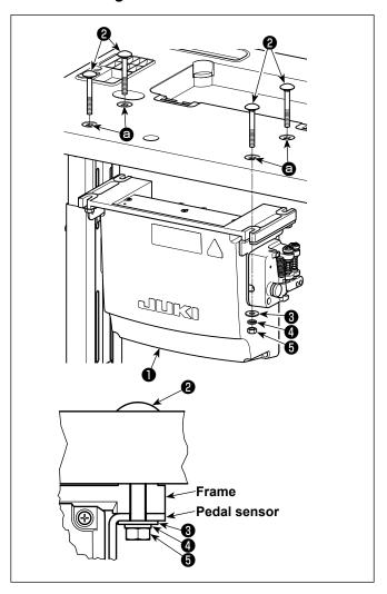
Install control box ① on the table using four holes ② in the table. Secure the control box with four bolts ②, four plain washers ③ , four spring washers ④ and four hexagonal nuts ⑤ supplied with the control box. At this time, insert the nut and washer supplied with the unit as accessories as shown in the figure so that the control box is securely fixed.
