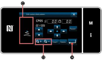
7) When **Q+Q- B** is pressed, the display size of pattern display area **O** is changed over.
