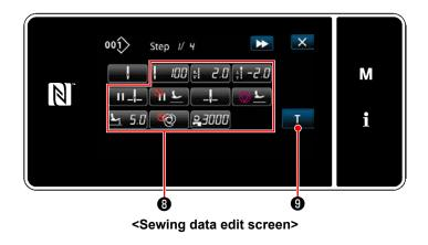
5) Setting other sewing data 3. The type of sewing data displayed on the "sewing data edit screen" changes according to the step changeover reference selected in the aforementioned item number 3. (See the table shown below.)
