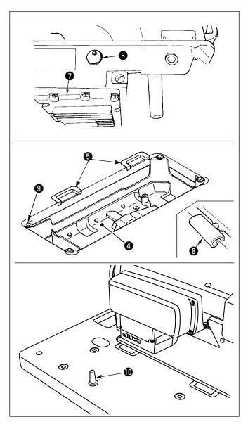
3) Remove air vent cap **6** attached to the machine bed. (Be sure to attach cap **6** when transporting the machine head in the state that the machine head is removed from the machine table.)
