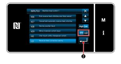
In the case the function item i51 or beyond is selected, the operation to be carried out when the button is pressed is set.
