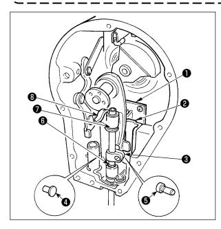
It is effective to periodically replenish the grease using the exclusive grease (grease tube part No.: 40006323) supplied as accessories. (It is not necessary to replenish the grease when the sewing machine is operated under the normal condition. However, when the sewing machine is operated under the severe condition, perform replenishing.)
