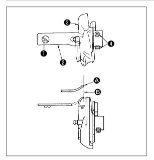
When you replace the sewing hook, remove it in the following procedures;
