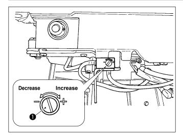
Adjustment of the amount of oil in the hook is performed with oil amount adjustment screw ①.
