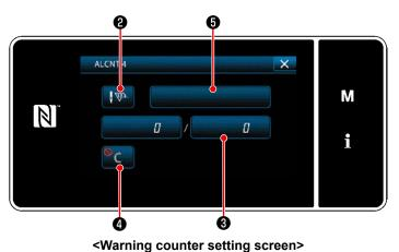
4) When is pressed, the "warning counter type selection screen" is displayed.
