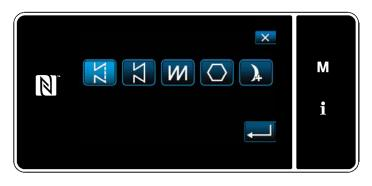
Select the sewing pattern (free stitching, constant-dimension sewing, overlapped stitching, polygonal-shape stitching, continuous sewing).
