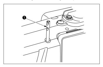
Insert needle thread guide pin **1** into the slot on the machine head.
