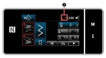
2) Pour oil into the oil tank unit until empty mark displayed on the upper right portion of the operation panel changes from Normal to Full.
