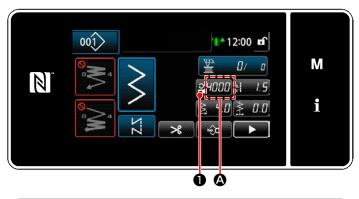
The sewing speed is displayed in section **(A)** on the panel. (Example of display: 4,000 sti/min)
