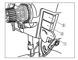
Various operations can be allocated to hand switch ① and machine head switches ② and ③.
