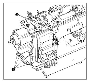
14) Attach the INT PCB and presser motor base in place with screws **1** and **2**.
