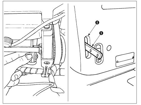
Insert reverse feed lever plate (asm.) B (3) that you have assembled in Step 2) from under the bed. Position reverse feed lever plate (9) so that it juts out from reverse feed lever hole (8) in the arm.
