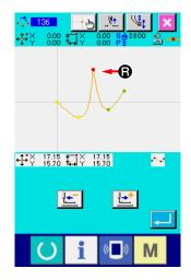
When you desire to move point **3** to point **3**, the result will be changed by selecting either shape point of rear **2** or front **3**.
