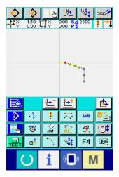
The pattern data subsequent to the deleted point(s) does not move but the pattern data before and after the deleted point(s) are joined by jump feed.
