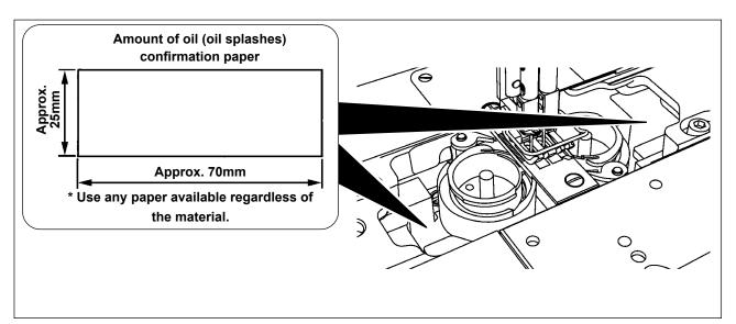
\* In the case of measuring the oil quantity in the hook, measure it under the "Bobbin winding mode".
