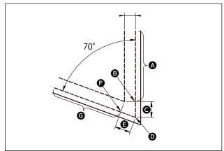
In the case of carrying out the corner stitching at the angular portion as illustrated in the figure, set the steps as described in the table shown below.
