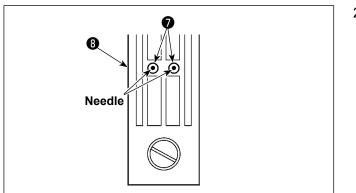
2) Replace the feed dog and throat plate with those for the bottom feed. Then, adjust the position of needle rocking rod fixed base **4** so that the center of the respective needles is aligned with needle holes 🕖 in throat plate (3). Then, tighten setscrew (5). Then, replace the presser foot with that for the bottom feed.
