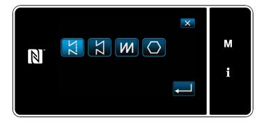
Select a sewing pattern (free stitching, constant-dimension sewing, overlapped stitching or polygonal-shape stitching). 2 Confirming the data on the created sewing pattern
