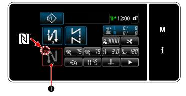
The sewing-end reverse feed stitching pattern can be operated when the sewing-end reverse feed stitching function is placed in the ON state( mark is not displayed). If this function is placed in the OFF state press the sewing end reverse feed stitch button to switch off mark display to enable the sewing-end reverse feed stitching function.
