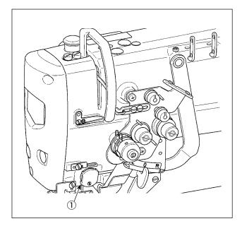
As same as the conventional wiper device, the thread clamp device is able to roll in the needle thread on the wrong side of material.
