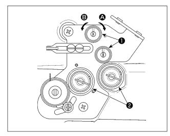
Turn thread tension nut No. 1 ① clockwise ② to shorten the length of thread remaining on the top of needle after thread trimming. Turn the nut counterclockwise ③ to lengthen it.
