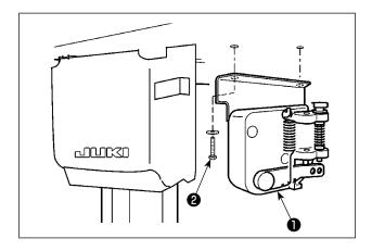
Secure pedal sensor ① to the table with two plain washers and two wood screws ② both of which are supplied with the electrical box.
