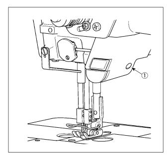
\* This LED is intended to improve operability of the sewing machine and is not intended for maintenance.
