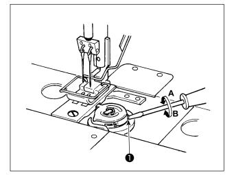
The bobbin thread tension is increased by turning bobbin thread tension screw ① clockwise A, or is decreased by turning it counterclockwise B.
