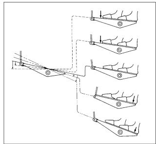
When you depress the pedal, the sewing machine starts sewing.
