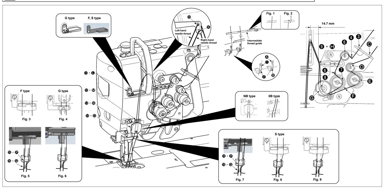
Thread the machine head following the order as illustrated in the figure.
