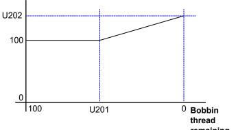
thread remaining amount [%]  Set "U201 Bobbin thread remaining amount for starting correction" with numeric keypad ①.
