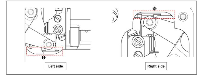
3) Remove dust accumulated in grooves \$9\$ and \$10\$ between the backward end position of the moving knife and the bed with a pair of tweezers or small tool in the downward direction. Check to make sure that the moving knife can move smoothly to its backward end.
