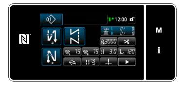
Four different types of counters are available; bobbin thread counter (left), bobbin thread counter (right), sewing counter, pitch time counter.
