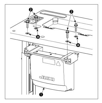
Install electrical box ① to the table by fixing four accessory bolts ②, which are supplied with the electrical box, in holes ③ in the table.
