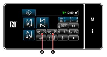
5 S005. Needle thread terraiker (right) 75 M i i 5 Active tension **2** permits setting of the needle thread tension on the operation panel according to each sewing condition. In addition, the data can be stored in memory.
