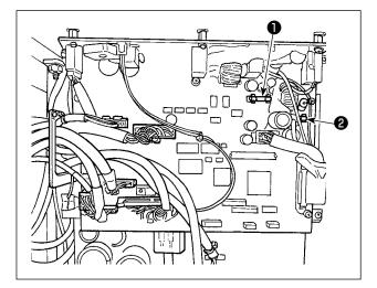
The machine uses the following two fuse. Both are the same fuses.
