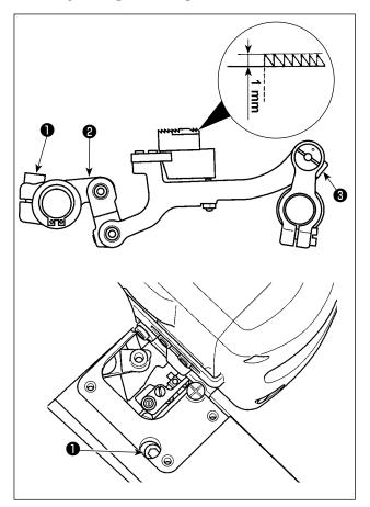
The standard height of the feed dog is 1.1 mm for the G type model, or 1.0 mm for the F and S type model, at its highest point above the throat plate.
