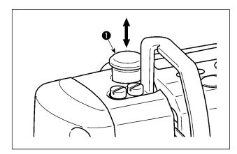
When the power to the sewing machine is in the OFF state, the presser foot can be lifted / lowered by moving presser bar cap **①** up or down by hand. Carry out this procedure for changing the gauge or adjusting the needle entry area.
