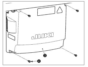
For the purpose of preventing the cord breakage, take care not to allow the cords to be caught between the control box and control box cover when attaching the latter.
