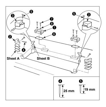
Attaching the hinge seats and the support rubbers of the machine head
