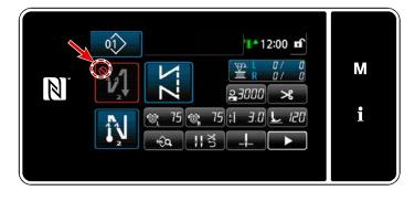
The sewing-start reverse feed stitching pattern can be operated when the sewing-start reverse feed stitching function is placed in the ON state mark is not displayed). If this function is placed in the OFF state, press the sewing start reverse feed stitch button to switch off mark display to enable the sewing-start reverse feed stitching function.
