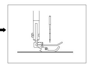
4) Place the multi-layered section of material under the presser foot, and press  $\mathbf{0}$ .
