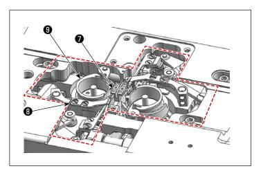
2) Remove dust accumulated on feed dog
