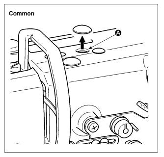
Remove the rubber cap, take out the felt in
