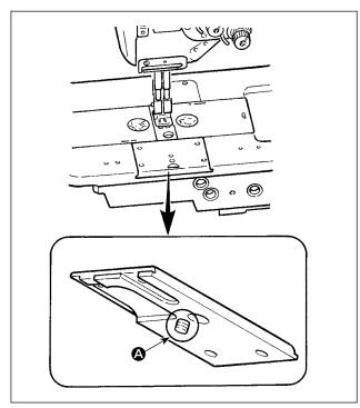
Be careful that screw (2) does not protrude in the rear of the bed slide when fixing the attachment to the bed slide with the screw.
