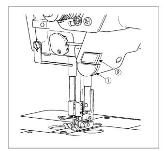
Various kinds of operations can be carried out by operating machine head switch (1) and hand switch (2) .
