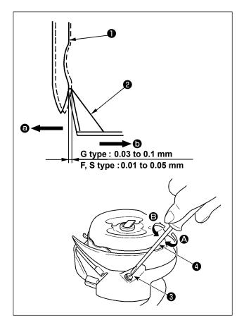
After you have changed the hook, check the position of the needle guard.
