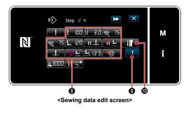
5) Setting other sewing data (3). The type of sewing data displayed on the "sewing data edit screen" changes according to the step changeover reference selected in the aforementioned item number 3. (See the table shown below.)
