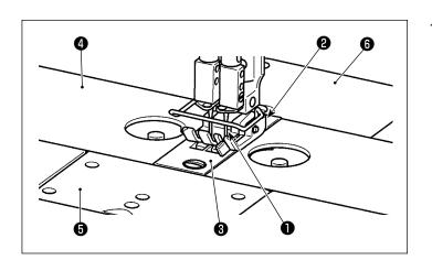
Detach needle ①, presser foot ②, throat plate ③, bed slides ④ (two pieces), attachment plate ⑤ and rear cover
