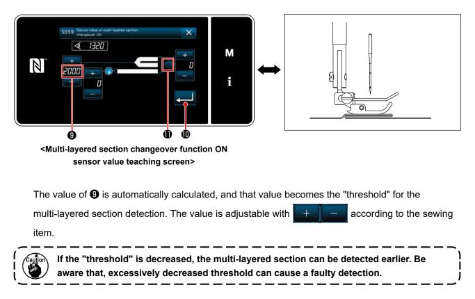
Press **1 1** is pressed, the "multi-layered section changeover function ON sensor value screen" is displayed.
