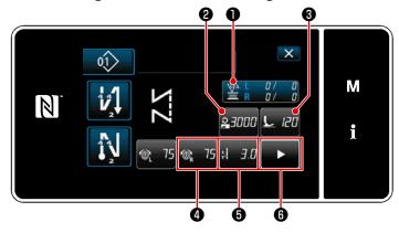
When one of the buttons **2** to **3** (**2** to **6** for the operator mode or cycle mode), the "Key customization selection screen" is displayed.
