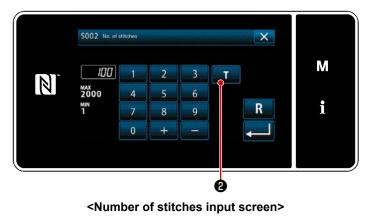
Press **①** on the sewing data list screen. Then, the number of stitches input screen is displayed.
