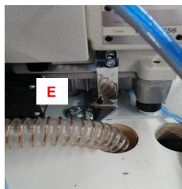
**3.2) Connecting the air tube to the air regulator. 3.3) Connecting the power supply**
