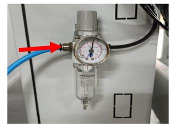
3.6) Connect the air tube to the air regulator.
