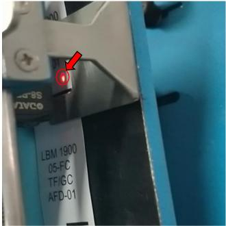
Turn the adjustment screw left or right to move the sensor point to the white (blank) area of the label.
