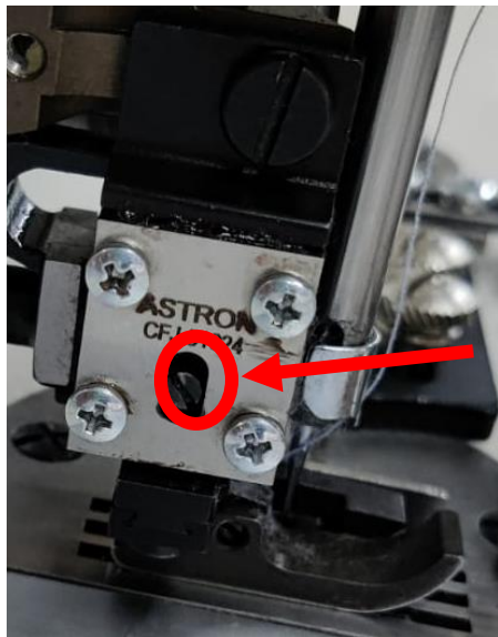
Step 3 : Center the screw in the slot
