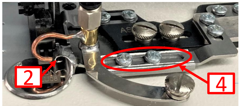
Step 2 : Remove the presser foot from the gauge
