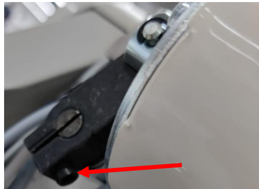
Step 4 : Tighten the screw with a little play in the direction of rotation.
