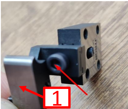
Step 1 : Remove the screw
