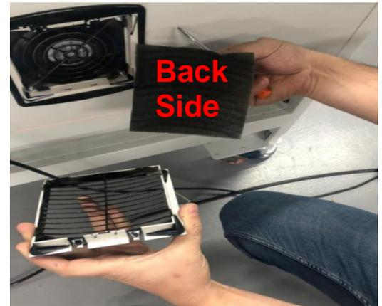
Open the cover of the air filters cover and take out the felts. Air filter can be cleaned with the compressed air gun.
