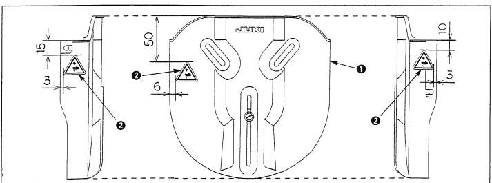
1) Put the warning seals 2 (three) on the stated position on the motor pulley cover 1.
