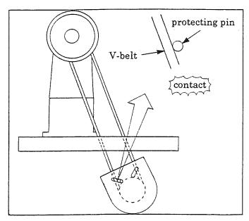
With this sewing machine, if you use the protecting pin of the motor pulley cover, V-belt will come in contact with the motor pulley cover.
