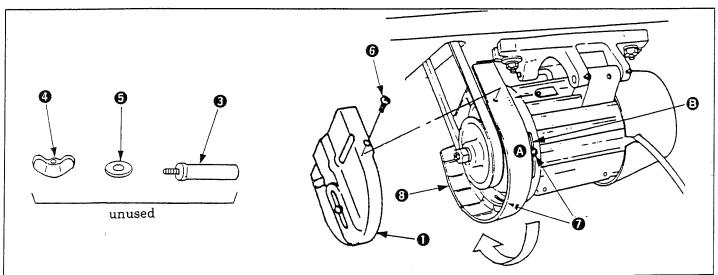
Without using the protecting pin 3, screw 4, washer 5, attach the motor pulley cover 1 using screws 6 (two). (You need not attach and adjust the protecting pin described in the Instruction Manual supplied with the machine.)
