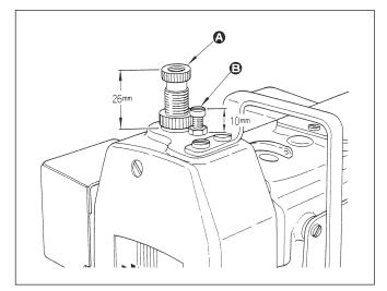
The pressure of walking foot (height of adjustment screw (2): Standard 26 mm) or the presser foot (height of the adjustment screw (3) Standard 10 mm) can be adjusted in accordance with the type of sewing product to be used.
