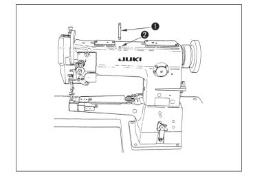
Insert take-up thread guide rod **1** attaching section is tapered of into attaching hole **2**.
