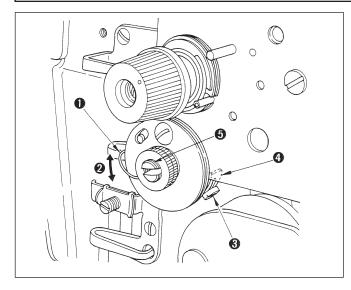
Adjusting the needle thread tension
