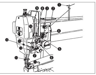
(For the DSC-245-7,DSC-245V-7) Thread the machine head in the order of ① through to ① . (Caution) Be sure to pass the thread through the left-hand side of
