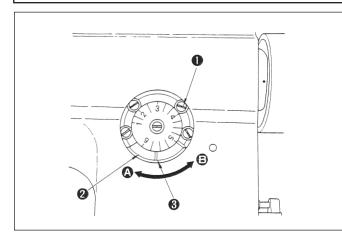
The seam ratio of forward stitch and reverse stitch is adjusted to be 1:1,but sometimes it shifts according to the sewing condition.
