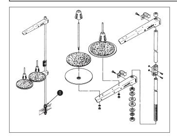
1. Assemble the thread stand, and insert it in the hole in the machine table, and fix it by tightening nut ①.
