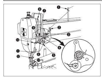
(For the DSC-245,DSC-245V) Thread the machine head in the order of ① through to ⑧ .
