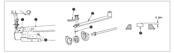
Feed dog ③ is factory-adjusted to jut out 0.8 mm from the surface of throat plate ① . How to adjust the height of the feed dog.
