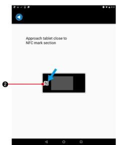
3) Approach the tablet close to the NFC mark ② on a panel. Once the terminal registration is successfully completed, the massage "Terminal is successfully registered" is displayed. \*When the transmission is not successful, an error message is displayed.
