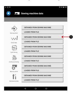
1) Press "OBTAINED FROM SEWING MACHINE" **1** button for the vector data.
