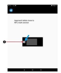
2) Approach the tablet close to the NFC mark ② on a panel.
