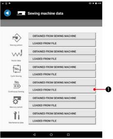
1) Press "OBTAINED FROM SEWING MACHINE" button **1** for the continuous sewing data.
