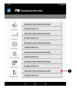
1) Press the "OBTAINED FROM SEWING MACHINE" button **1** of Maintenance data.
