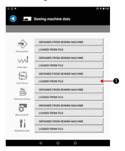
1) Press "OBTAINED FROM SEWING MACHINE" button **1** for the cycle sewing data.
