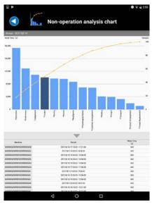
2) The non-operation analysis chart screen is displayed. Time taken by wasted work and the accumulation ratio of wasted work can be viewed on the non-operation analysis chart.
