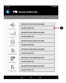
1) Press the "LOADED FROM FILE" button **①** of Sewing pattern.
