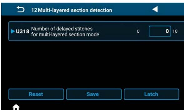
When approaching a multi-layered section, depending on the sewing conditions, the mode may switch to multi-layered section mode before the multi-layered section is reached.
