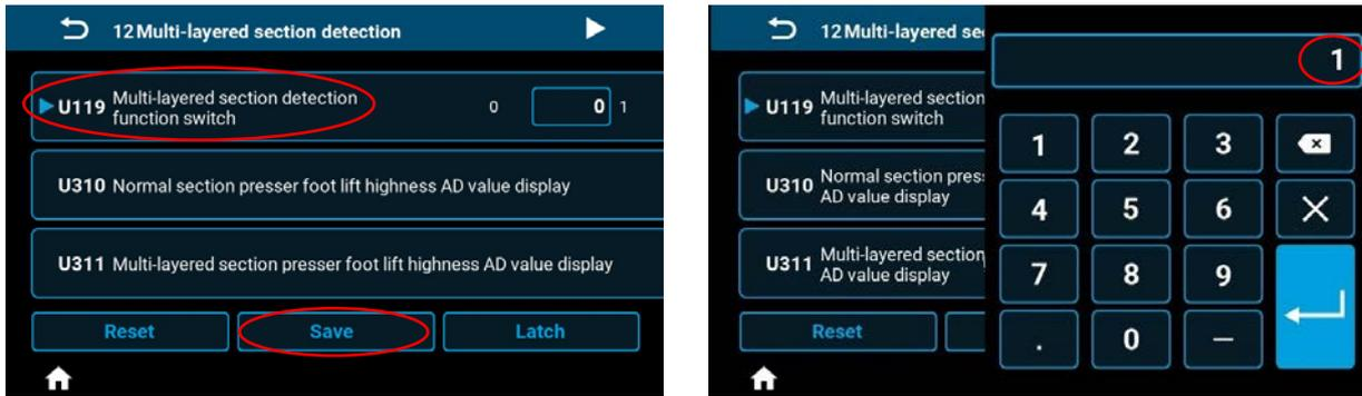
**Caution** If you select “8: One touch utility changeover function” for U015 “Hand switch A function setting” or U174 “Hand switch B function setting”, you cannot set U119 “Multi-layered section detection function setting” to 1.
