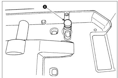
10) Attach the under-cover to the table. Place knee-lifter push rod 4 to the table.
