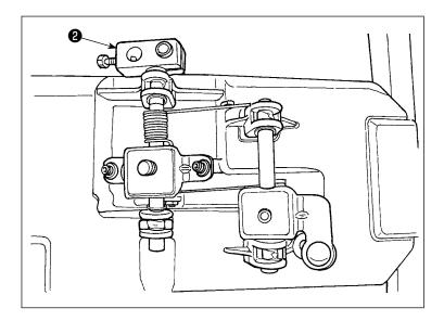
9) Secure knee-pad vertical shaft mounting arm (asm.) 2 .
