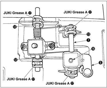
8) Insert knee-lifter actuation arm 3 and knee-lifter rotation arm setscrew 16 through the hole in knee-lifter operating shaft 2 and secure them.
