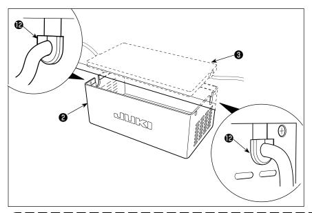
9) Fit reactor cover **2** over reactor base asm. **3** .
