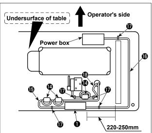
11) For two ring cores **(!**), clamp the power cord of the electrical box after winding the cable round the torus of the ring core twice.
