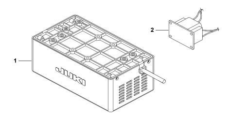
When using the following, refer to "2-6. Installing the reactor box [Only for the EU type models]" p.5 or "2-6. Installing the reactor box (Only for EU type models)" in the Instruction Manual for the DDL-8000AS, AB.
