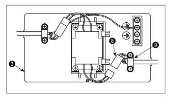
6) Secure power cord asm. 3 coming from the electrical box to reactor base asm. 3 with bundled wire clamp 9.
