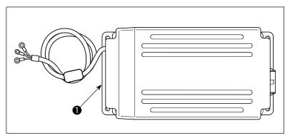
1) Remove the reactor box **1** from the accessory box.
