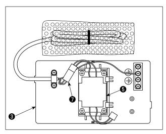
4) Connect the connector 7 of the power cord that is fixed to reactor base asm. 3 to the connector of reactor 5.
