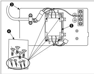
5) Take out wood screws (ST4.2 x 25) from screw bag 4. Secure reactor base asm. 3 and reactor
