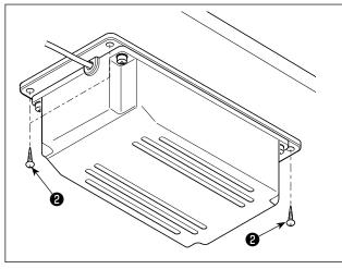
2) Remove the wood screws ② from the accessory bag and install the reactor box under the table.
