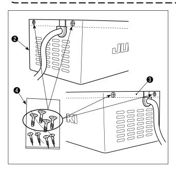
10)Take out reactor cover fixing screws from screw bag 4 . Secure reactor cover 2 to reactor base asm. 3 with the fixing screws (at four locations).
