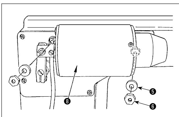
7. Install solenoid (asm.) 8 with washer 5 and nut 6.
