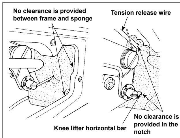
4. Make sure that a sponge is placed as illustrated in the figure. If not, pass the tension release wire in the upper notch and pass the knee lifter horizontal bar in the lower notch so that no clearance is provided in the notches. In addition, make sure that there is no clearance between the frame and the sponge.
