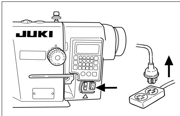
1. Press the OFF button of the power switch to turn OFF the power after confirming that the sewing machine has stopped.
