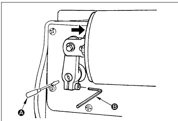
8. Lower the presser foot until it comes in close contact with the throat plate. Turn solenoid shaft counterclockwise with a screwdriver A with the solenoid pressed in the direction of the arrow, then tighten the connecting stud clamping screw with hexagonal wrench key B.
