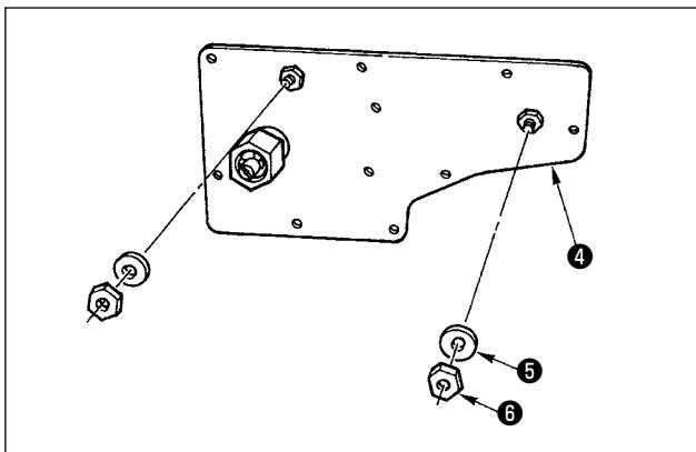
5. Remove washer 5 and nut 6 from side plate (asm.) 4 of the device.
