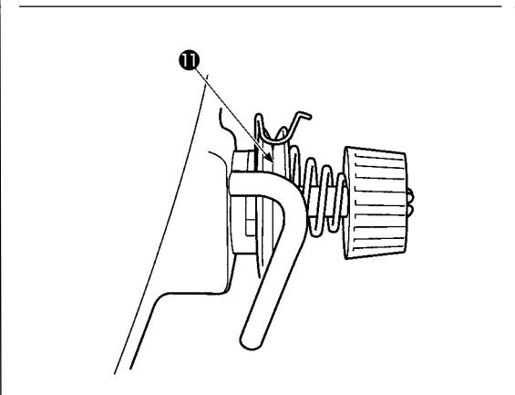
**11. Adjustment of the floating amount of the tension disc No. 2.**
