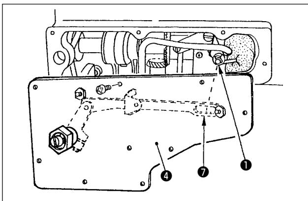
6. Install side plate (asm.) 4 on the sewing machine. At this time, install side plate (asm.) so that the slot in solenoid link 7 fits over knee lifter horizontal bar pin 1.
