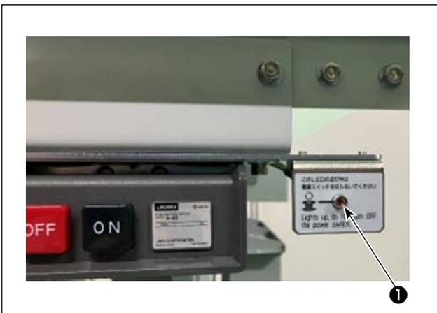
Lamp ❶ mounted next to the power switch indicates that the device is in operation.
