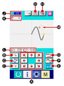
The figure on the right-hand side is the position specifying screen which is displayed when specifying the position at the setting of function. The selected function code is displayed at **①**.
