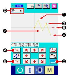
The breakpoint is the point where two points of the shape point of spline sewing are overlapped, and shows the termination of one spline curve. The point where ENTER button DECIDING POINT button Spline sewing becomes the breakpoint.
