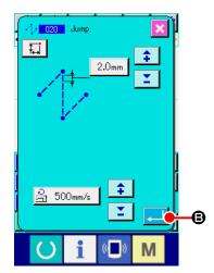
Press ENTER button **E** in the jump feed setting screen to display the jump feed position specifying screen.
