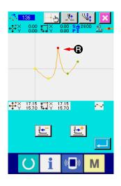
When you desire to move point (3) to point (5), the result will be changed by selecting either shape point of rear (2) or front (3).
