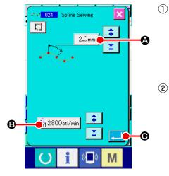
**Display the spline ordinary sewing setting screen.** When selecting and executing SPLINE ORDINARY SEWING (function code 024) in the code list screen, the spline ordinary sewing setting screen is displayed.
