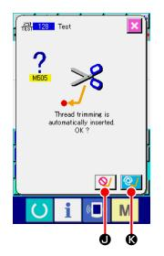
In the case where the thread trimming command does not exist in the termination of pattern and before jump feed, the automatic thread trimming insertion confirmation screen is displayed after pressing SEWING PREPARATION button  $\square$ , and whether inserting thread trimming  $\bigcirc$  or not  $\bigcirc$  can be selected. When either one of the buttons is pressed, the screen moves to the trial sewing preparation screen. 1. When performing the trial sewing, input data
