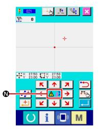
At **(a)** warning pictograph **(b)** is displayed when setting possible range is exceeded or the like.
