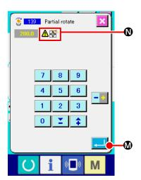
When a rotation angel is entered on the angle numeric-value input screen and ENTER button  $\checkmark$  is pressed, the work clamp move confirmation screen is displayed. At this time, the work clamp moves along with the rotation angle. If the rotating object exceeds the sewing area when it is rotated,  $\land$  is displayed.
