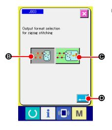
Selecting the zigzag sewing output method. The zigzag sewing output method is displayed. Select
