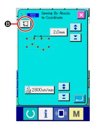
Changeover between the relative insertion and the absolute insertion can be conducted on sewing item setting screen  $\boldsymbol{\Theta}$ .
