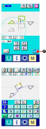
After inputting a rotation angle, press ENTER button When the ENTER button is pressed, the pattern rotates and the screen returns to the standard screen.
