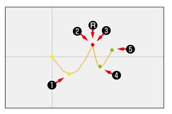
When performing the shape point deletion of either point of rear **2** or point of front **3**, the breakpoint becomes the normal passing point and the continuous spline sewing is formed.
