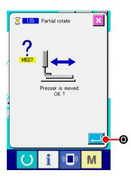
When ENTER button move confirmation screen, the work clamp moves to the position which corresponds to the rotation angle. Then, the screen returns to the rotation angle specifying screen.
