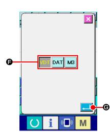
Select the kind of pattern to read in from vector format VDT standard format **DAT**, and writing style data M3 of (). The color of the selected button is changed When ENTER button **C** is pressed, the setting has been
