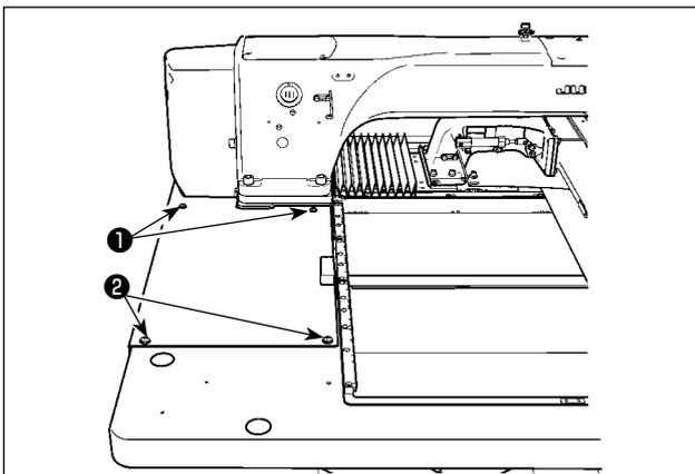
1) Remove screws ① and ② to remove the cover.
