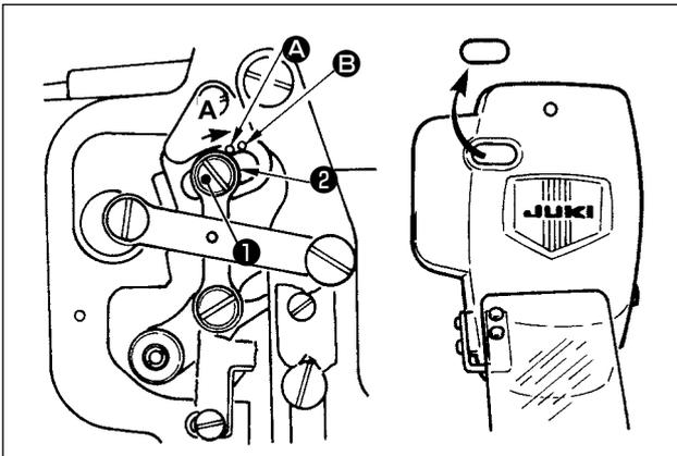
\* Turn ON the power once, and turn OFF the power again after making the intermediate presser in the lowered state.
