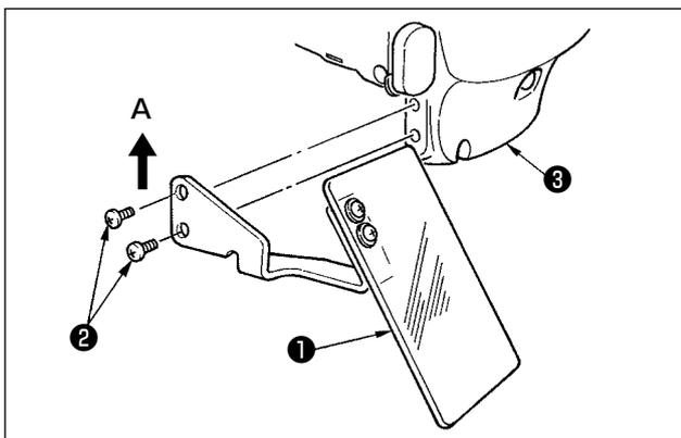
Use eye protection cover ① after securely attaching it on face plate cover ③ with screw ② .
