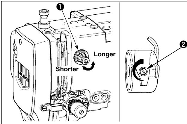
If thread tension controller No. 1 **1** is turned clockwise, the length of remaining thread on the needle after thread trimming will be shorter. If it is turned counterclockwise, the length will be longer. Shorten the length to an extent that the thread is not slipped off.
