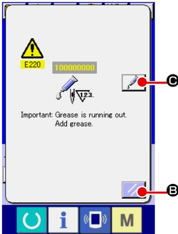
When the sewing machine has been used for a certain number of stitches, error "E220 Grease-up warning" is displayed. This display informs the operator of the time of replenishing the designated places with grease. Be sure to replenish the places with the grease below. Then call the memory switch U245, press CLEAR button
