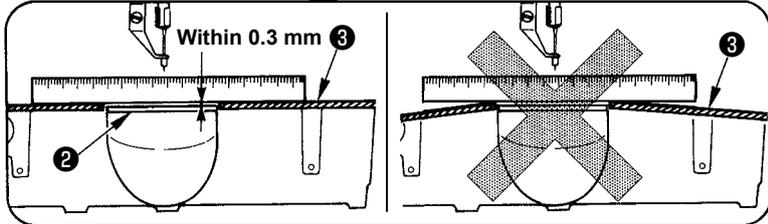
1. Fix the throat plate auxiliary cover ③ so that is higher than the throat plate ② (within 0.3 mm). When it is lower than the throat plate ②, needle breakage or the like due to the defective feed will be caused.
