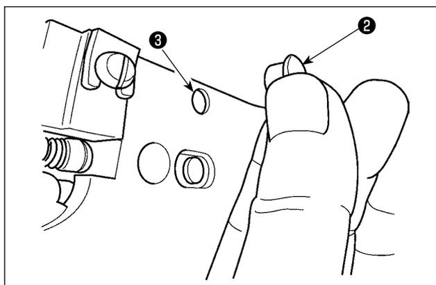
When thread is caught at top end ① of the thread clamp, thread clamp becomes incomplete and sewing trouble at the sewing start will be caused. Thread waste and lint are likely to accumulate in the sections which are shown in the circles. The sections should therefore be periodically cleaned by removing the throat plate and by blowing air through hole ③ by removing rubber plug ② .
