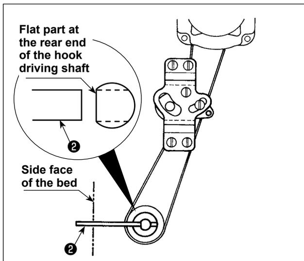
2) Face the flap section of the rear end of hook driving shaft to the frame side, and insert hook driving shaft positioning shaft ② (13704705) supplied with the machine as accessories from the hole on the machine bed side.
