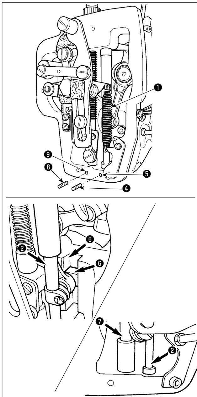
1) Open the frame cover to remove intermediate presser auxiliary spring B ① .
