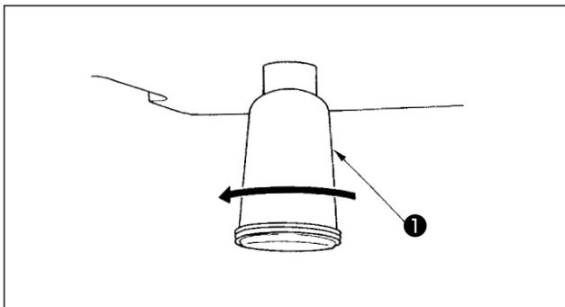
When polyethylene oiler ❶ becomes filled with oil, remove polyethylene oiler ❶ and drain the oil.
