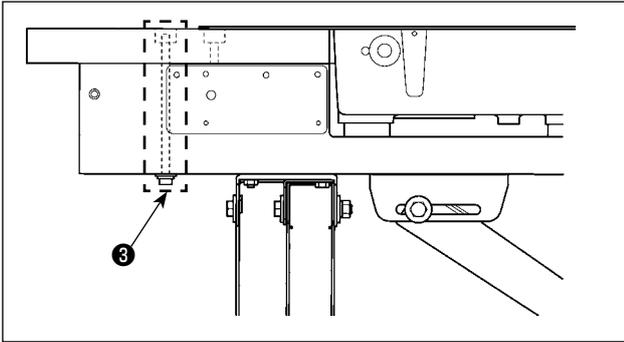
2) Remove table fixing bolts ③ which are mounted at two locations of the table stand.
