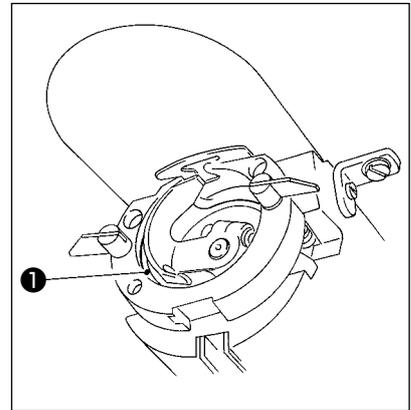
1) Check that the place between lower line **B** and upper line **A** is filled with oil. Fill there with oil using the oiler supplied with the machine as accessories when oil is short.
