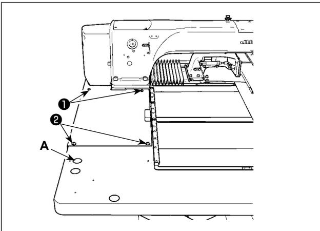
4) Temporarily fix table fixing bolts ③ at two locations from the table stand side.
