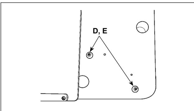
9) Secure the operation panel stoppers (accessory D) in the punched locations at near side of the right table using wood screws (accessory E).
