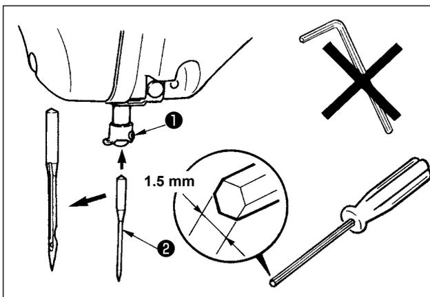
Loosen setscrew **1** and hold needle **2** with the long groove facing toward you. Then fully insert it into the hole in the needle bar, and tighten setscrew **1**.
