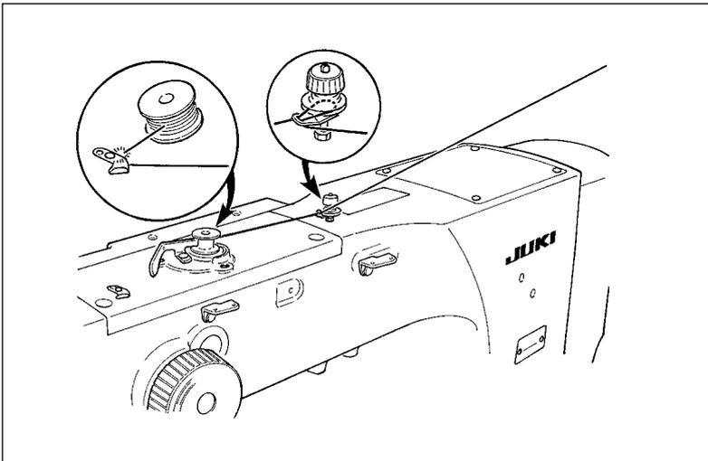
Thread the bobbin winder and wind the bobbin thread onto the bobbin as illustrated in the figure.
