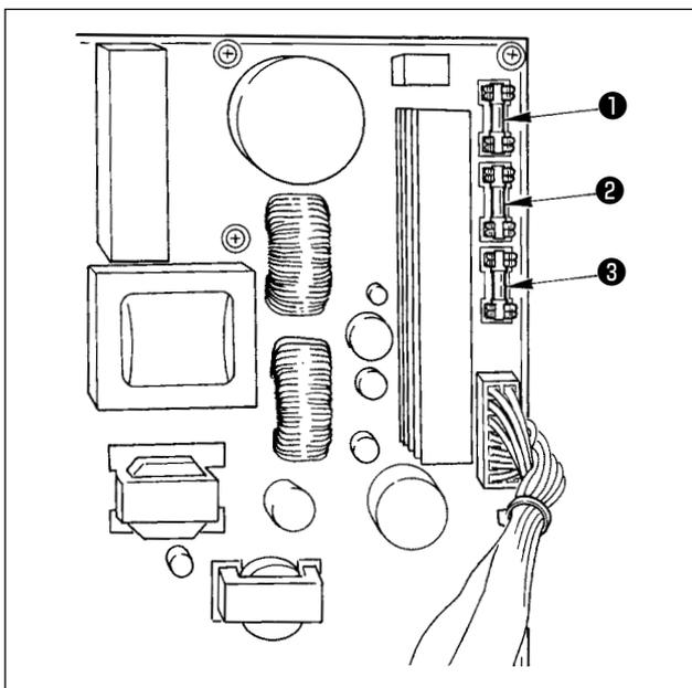
The machine uses the following three fuses :
