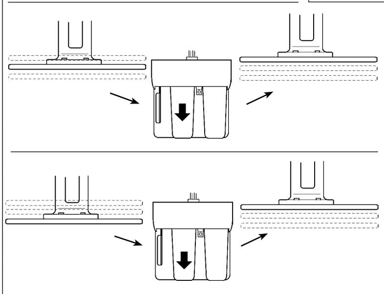
④ When depressing 1st step of the intermediate pedal again in the state that the presser is in the intermediate position, the presser goes up to the top.
