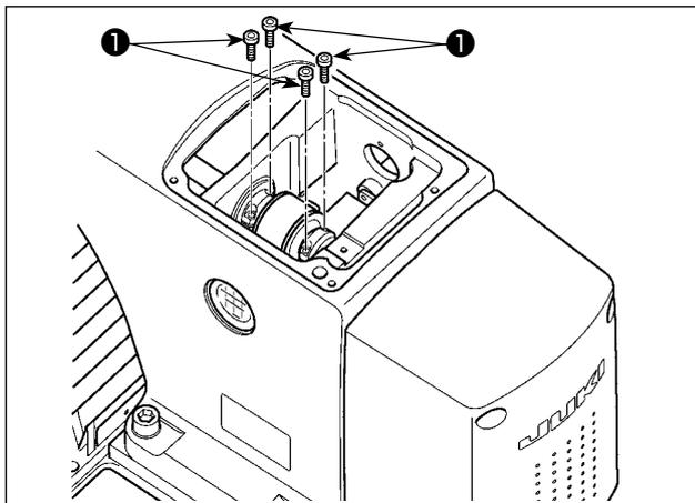
1) Loosen four main shaft sprocket setscrews ① .
