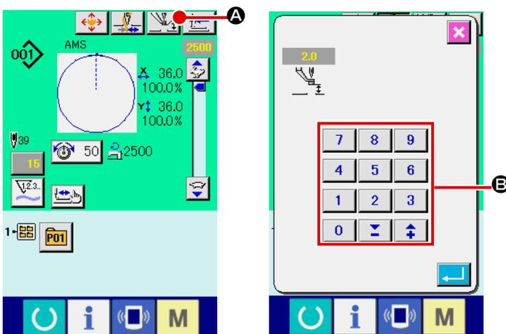
Press INTERMEDIATE PRESSER SETTING button **A** and adjust with TEN keys **B** so that the clearance between the bottom end of intermediate presser and the cloth is 0.5 mm (thickness of thread used).
