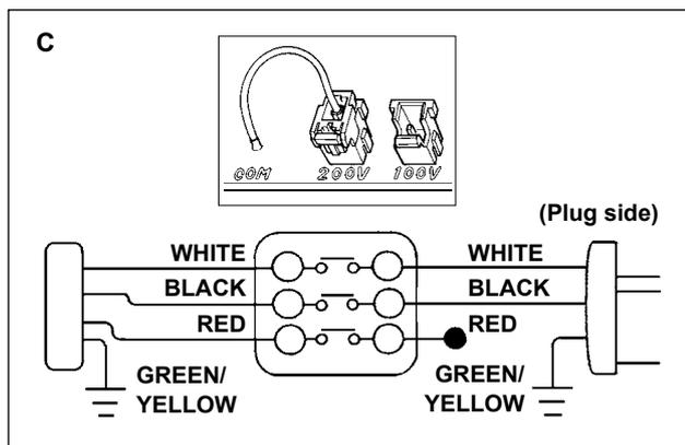
**(Caution) Securely perform the insulation treatment to the red terminal which is not used with insulation tape or the like. (When the insulation is insufficient, there is a danger of electric shock or leakage current.)**
