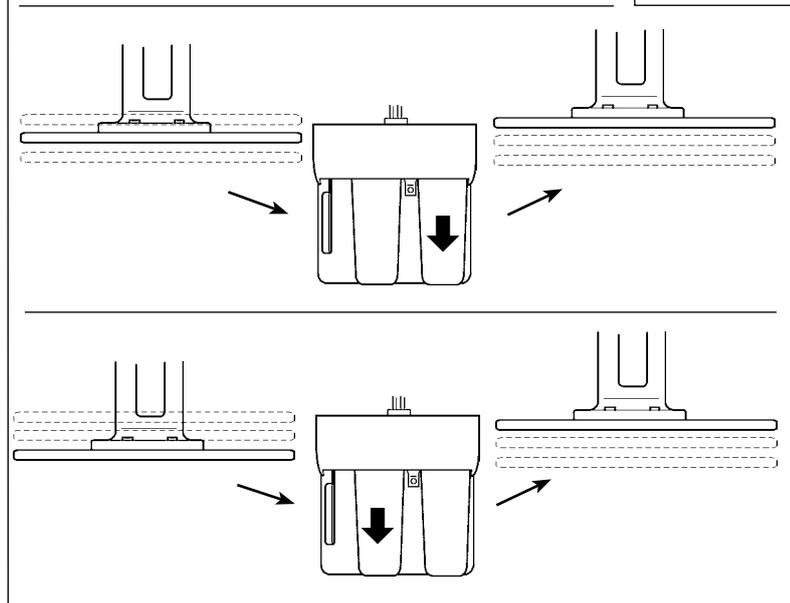
④ When re-depressing the right pedal in the state that the presser is at the intermediate position, the presser goes up to its upper dead point.
