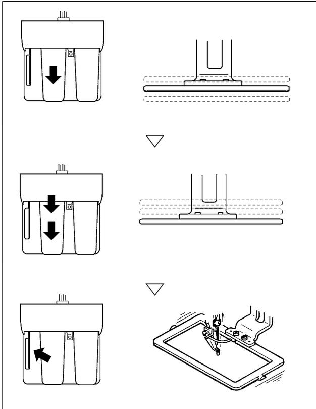
① When depressing 1st step of the intermediate pedal, the presser stops at the intermediate position.
