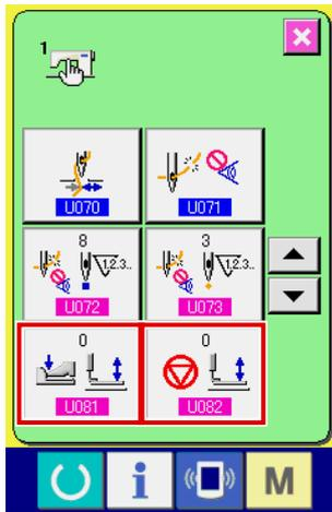
2-step stroke function can be used by changing setting of memory switches **U081** and **U082**.
