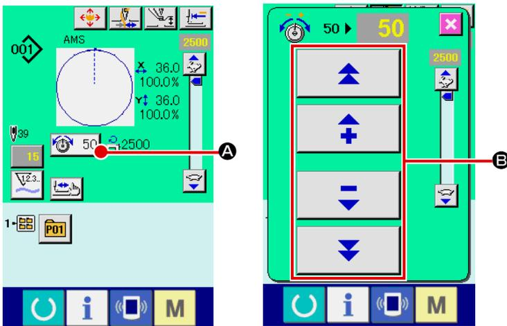
1) Select THREAD TENSION button **A** in the sewing screen.
