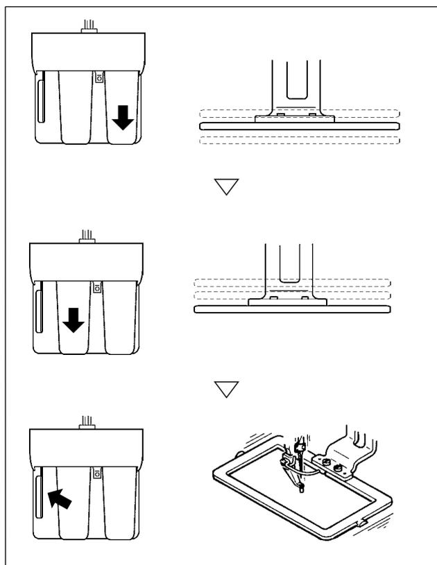
① When depressing the right pedal, the presser stops at the intermediate position.
