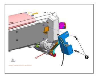
3) Remove the fixing screws **6** (two locations) of the intermediate presser cover of the sewing machine, install the mounting plate **4**, and fix with screws again to install onto the sewing machine.
