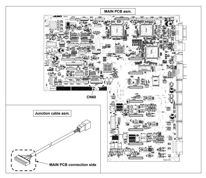
4) Open the electrical control box. Connect the junction cable (40105094) to the CN60 on the MAIN PCB.
