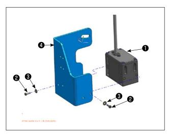
Install the bar code reader ① onto the mounting plate ② using the screws ② and the washers ③ (two locations) which are included as the accessories.
