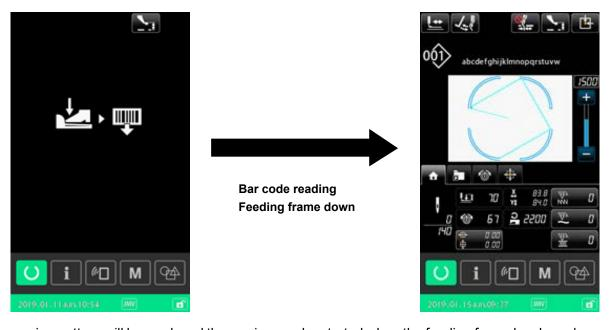
The sewing pattern will be read, and the sewing can be started when the feeding frame has been lowered.
