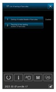
When you have enabled the bar code, the "BAR CODE READING POSITION TEACHING" button is displayed on the bar code setting list screen. Refer to "4-3-2. Fixed retraction position teaching" P.7 for how to use the bar code reading position teaching function.
