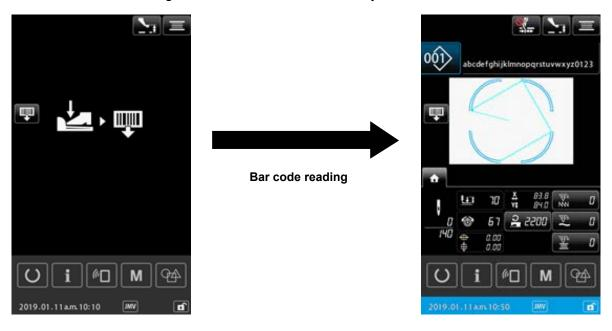
In the preparation state, trading on the work clamp foot switch (pedal) will initiate the actions of bar code reading, pattern reading and feeding frame down.
