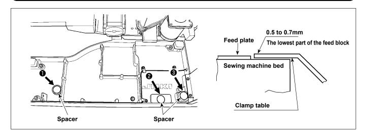
If the machine head comes down from its normal position due to aged deterioration, the folded edge of the material and the seam (the edge) may not be properly aligned when placing the material position on the machine head. In the case the smallest clearance (the difference in height) between the machine head bed and the feed section is 0.7 mm or more, place spacers (0.5 mm and 1.0 mm) at locations ①, ② and ③ to decrease the clearance (the difference in height) to 0.7 mm or less
