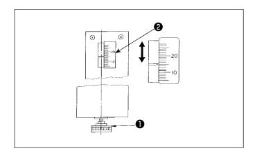
Check to be sure that the seam allowance is set to 21 mm. If not, adjust the seam allowance to 21 mm. Insert preset adjusting knob ① which is supplied in the tool box into the hole, and turn the knob to set the seam allowance to the value indicated by scale (21mm) marker ② . After the adjustment, return knob ① to the tool box to prevent it from being lost.
