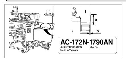
When moving the device after you have installed it in your plant, ground the device referring to the dimensions given on the attached sheet
