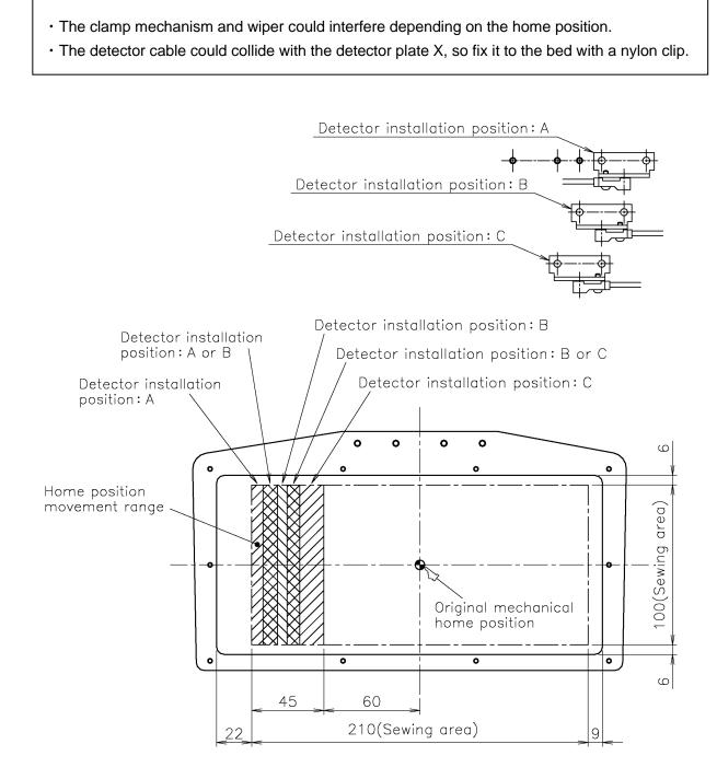
[Note] The shaded section below is the optimum range for moving the home position.
