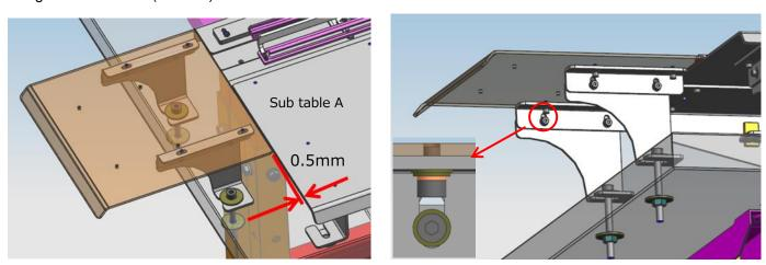
A clearance of approx. 0.5mm is needed between the sub table A and the feed plate.
