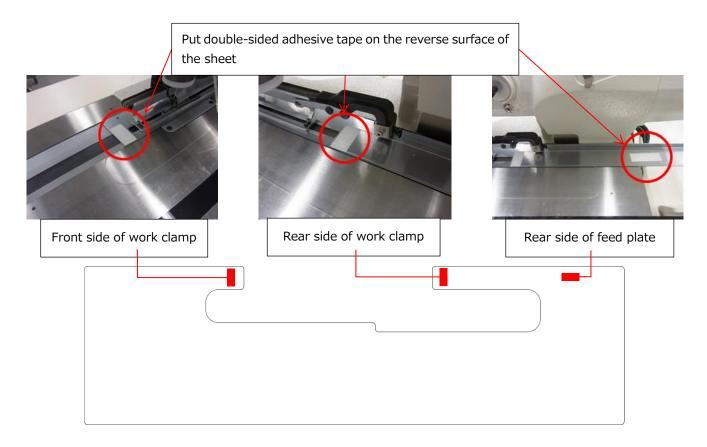
The feed plate slides smoothly by putting the slide assisting tape (1 piece) (40044824) supplied with the machine as an accessory on the undersurface of the feed plate.
