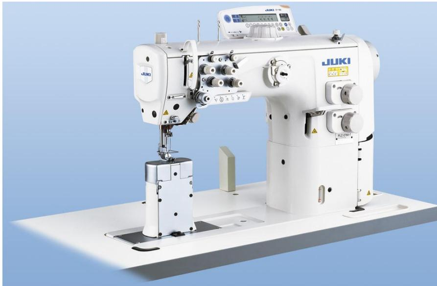
JUKI will release newly developed non-apparel machine “PLC-2700 series / Post-bed, Unison-feed, Lockstitch Machine with Vertical-axis Large Hook” which is best-suited for sewing the top stitches on the curved and 3D surface of Large and Heavy materials such as Car seats, Sofas and Sports Goods from June in overseas markets and from July in Japan.
