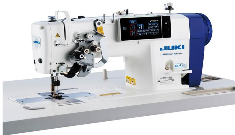
JUKI is going to launch the new semi-dry head, 2-needle, needle-feed, lockstitch sewing system for overseas markets from November, 2019. This sewing system is based on the 2-needle lockstitch machine and comes with digitalized "sewing" adjustment functions. Thanks to the digitalization, not only improved seam quality and shorter setup changing time are achieved, but also production management is enabled by interlocking JUKI exclusive application and the sewing machine.
