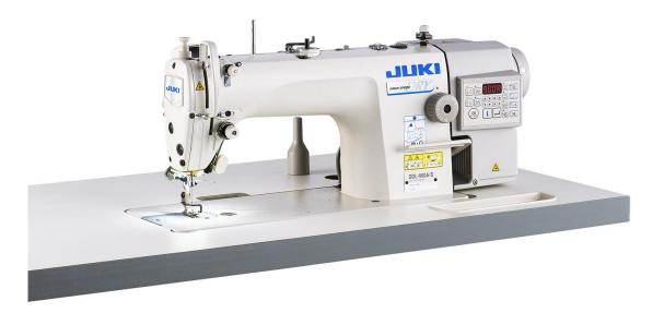
JUKI will launch the "DDL-900A" in overseas markets from December, 2014. This is a direct-drive, high-speed, 1-needle lockstitch machine which is provided with a newly-developed mechanism called the "DRY" Oil Pan System for preventing oil stains on sewing products.
