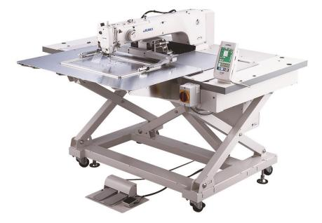
JUKI launches the "AMS-224EN4530R/AW-3", computer-controlled cycle machine with input function (full-rotary hook type, with automatic bobbin thread winding and feeding device) in overseas markets on the 21st of April. This new model is provided with automatic bobbin thread winding and feeding function. This function eliminates manual bobbin changing work, which causes interruptions of the production process, thereby increasing productivity.
