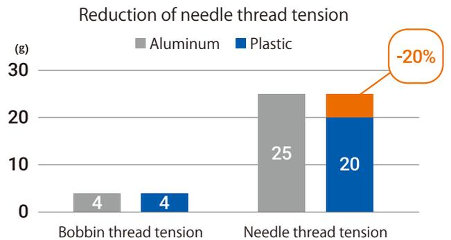
[Model used: LZ series (3,000rpm) / thread used: resilon thread #60 / bobbin thread tension: 4g]
