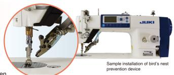
By automatically grasping the needle thread at the start of sewing and realizing the optimum amount of needle thread, it is effective for not only "improvement of quality at the start of sewing" but also "bird's nest prevention".
