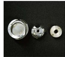
The non-rotary bobbin eliminates irregular stitches which have a tendency to occur at some sewing speeds and bobbin-thread tension fluctuations which have a tendency to occur according to the bobbin thread remaining on the hook. Since the bobbin thread is fed without rotating the bobbin, the bobbin never idles.
