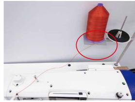
Put the thread inside the cone from the top, pass it through to the bottom, and use it by pulling it out from the thread groove of the base plate. The thread can be stabilized by passing through
