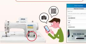
When the inspection launches, carry out the steps in sequence according to the instructions in the smartphone app.
