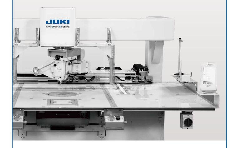
1-needle CNC sewing machine (head turning type) AMS-251
