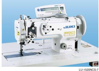
2-needle, Unison-feed, Lockstitch Machine with Vertical-axis Double-capacity Hook
