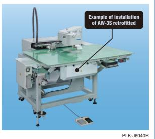
Automatic 1-needle Shoelace Loop Attaching Machine (Provided with a preset loader)
