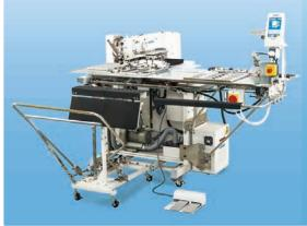
Computer-controlled Cycle Sewing Machine with Input Function (For sewing pockets on jeans) < With presetting device>
