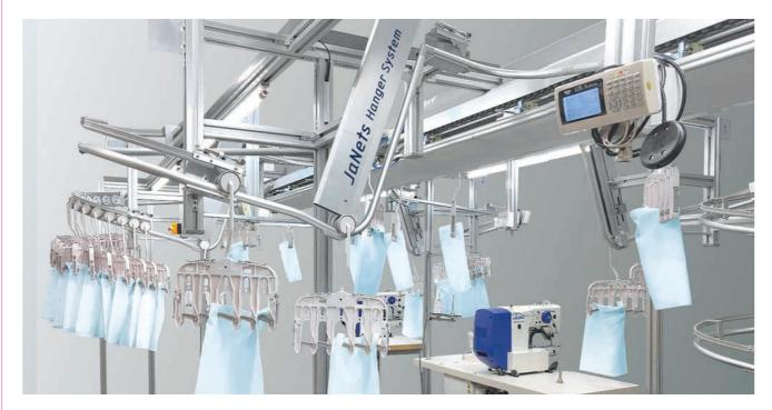
The JaNets hanger system does more than just transports products to the sewing station on hangers. Production progress of hanger lines can be obtained in real time from JaNets reports. The input amount for the assembly line can be examined based on the parts output managed by JaNets, preventing delays in the input of parts for the assembly line. JUKI offers the most suitable hanger system considering sewing items and factory facilities.
