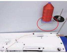
Put the thread inside the cone from the top, pass it through to the bottom, and use it by pulling it out from the thread groove of the base plate. The thread can be stabilized by passing through the narrow groove
