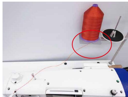
Put the thread inside the cone from the top, pass it through to the bottom, and use it by pulling it out from the thread groove of the base plate. The thread can be stabilized by passing through the narrow groove.
