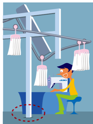
Stand type Set up and fix poles on the floor.
