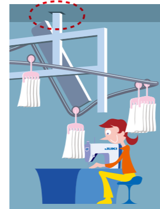
Ceiling type By hanging from the ceiling, there is no obstruction under the hanger system, so the equipment can be easily arranged.
