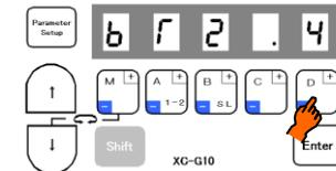
In the following table, the number of correction stitches "-1" corresponds to 4. Set [BT2] to 4. (This completes correction of the start tacking section.)
