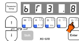
In the following table, the number of correction stitches "-2" corresponds to 8. Set [BT3] to 8. (The backward section now has three stitches. The forward section is increased to two stitches for a total of three stitches.) (Fig. 1)
